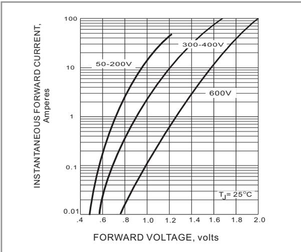
Fig.3 FORWARD CHARACTERISTICS
