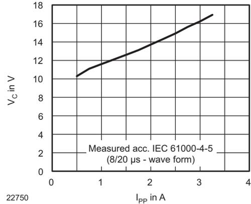
Fig. 4 - Typical Peak Clamping Voltage  $V_C$  vs.
