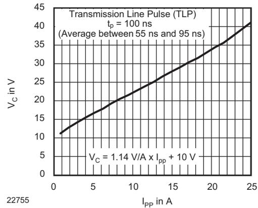
Fig. 5 - Typical Peak Clamping Voltage  $V_C$  vs.
