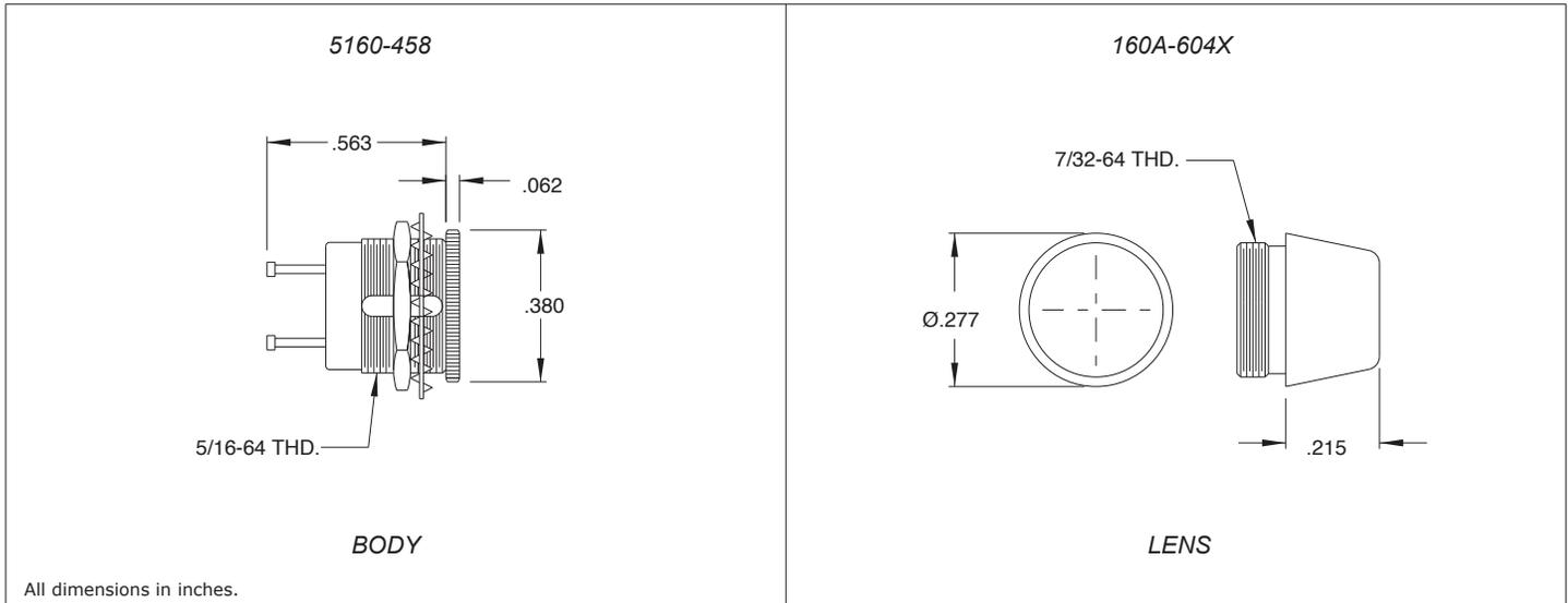
The Chicago Miniature Lamp Gemlite Indicator Light is a versatile design capable of accepting all T-1 sub-midget flange based lamps. These high quality indicators provide reliable service in a vast array of military and commercial applications where a miniature relampable front panel indicator is required. The lamp is not included with this indicator light. Please order the required lamp separately.
