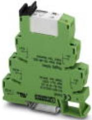
PLC-INTERFACE, consisting of PLC-BPT.../21-21 basic terminal block with push-in connection and plug-in miniature relay with power contact, for mounting on NS 35/7,5 DIN rail, 2 PDTs, input voltage 120 V AC/DC
