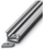
DIN rail, deep drawn, high profile, unperforated, 1.5 mm thick, material: aluminum, height 15 mm, width 35 mm, length 2000 mm
