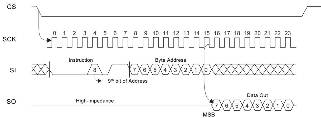
**Figure 7-7. WRITE Timing**
