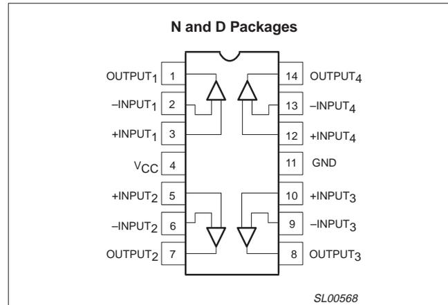
Figure 1. Pin configuration.
