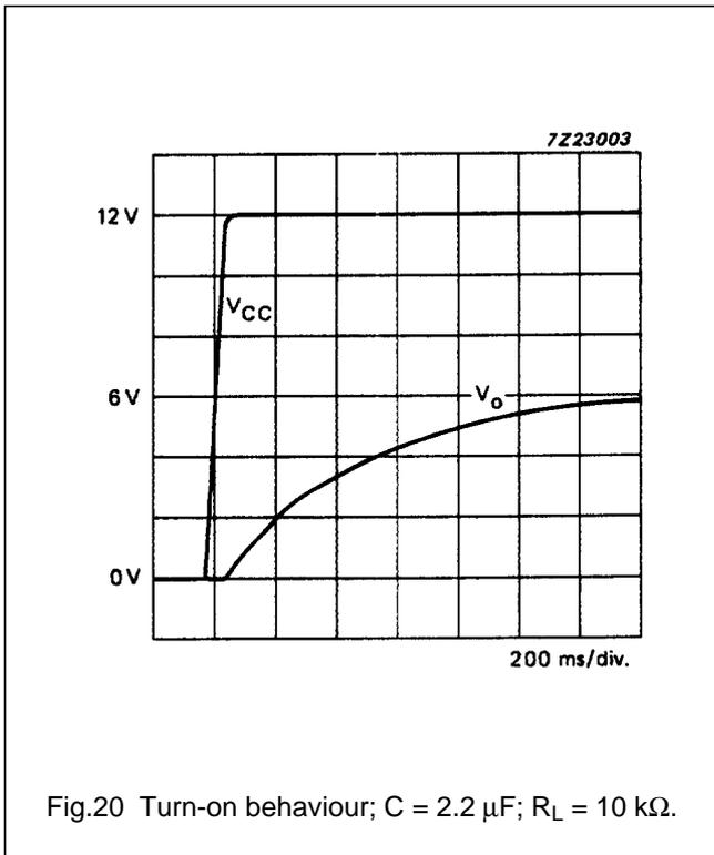
Fig.20 Turn-on behaviour;  $C = 2.2 \mu\text{F}$ ;  $R_L = 10 \text{ k}\Omega$ .
