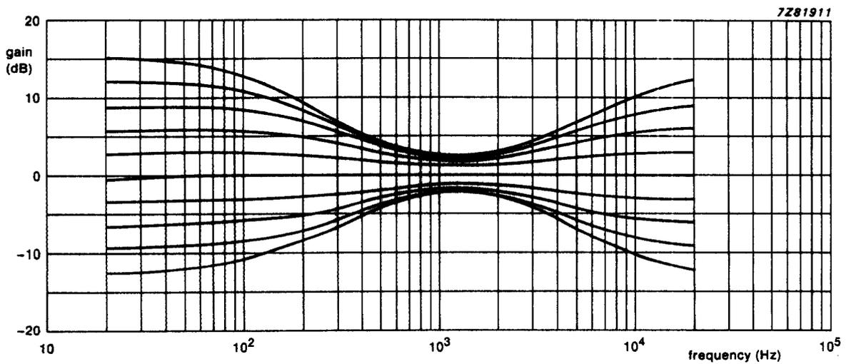
Fig.17 Frequency response of bass and treble control; bass and treble gain settings = -12 to +15 dB; gain is 0 dB;  $V_i = 0.1\text{ V}$ ;  $R_{S9} = 600\ \Omega$ ;  $R_L = 10\text{ k}\Omega$ ;  $V_{CC} = 12\text{ V}$ .
