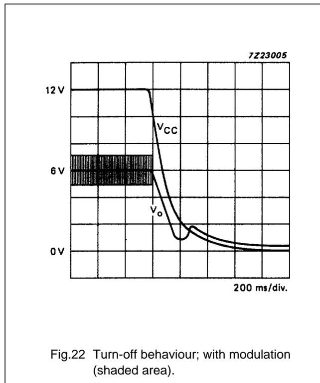
Fig.22 Turn-off behaviour; with modulation (shaded area).
