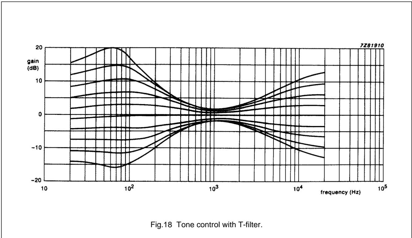
Fig.18 Tone control with T-filter.
