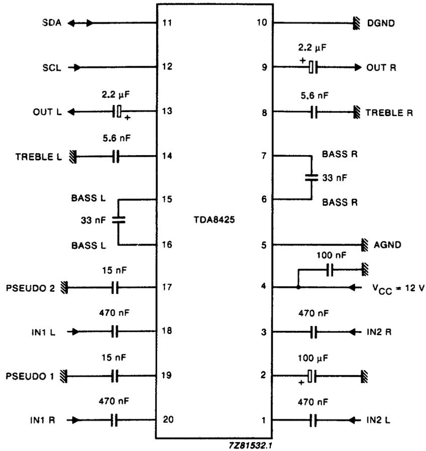
Fig.25 Test and application circuit diagram.
