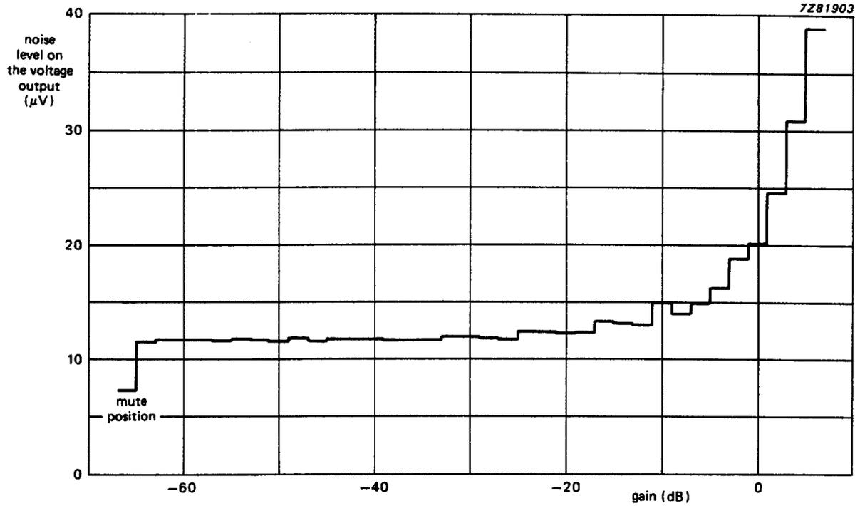
Fig.16 Noise output voltage as a function of gain; weighted CCIR468 quasi peak gain, + 6 dB to -64 dB;  $V_i = 0\text{ V}$ ,  $R_S = 0\ \Omega$ ;  $R_L = 10\text{ k}\Omega$ ; bass/treble = 0 dB;  $V_{CC} = 12\text{ V}$ .
