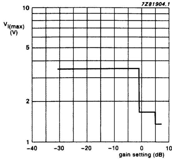
Fig.10 Input signal handling capability plotted against gain setting; THD = -60 dB; f = 1 kHz;  $R_S = 600 \Omega$ ;  $R_L = 10 \text{ k}\Omega$ ; bass/treble = 0 dB;  $V_{CC} = 12 \text{ V}$ .
