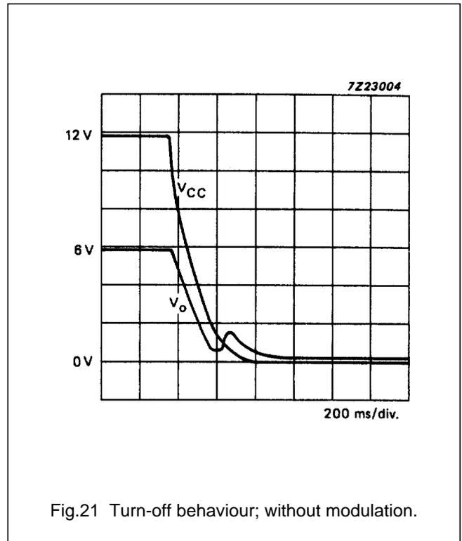
Fig.21 Turn-off behaviour; without modulation.
