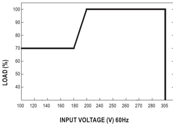
※De-rating is needed under low input voltage.
