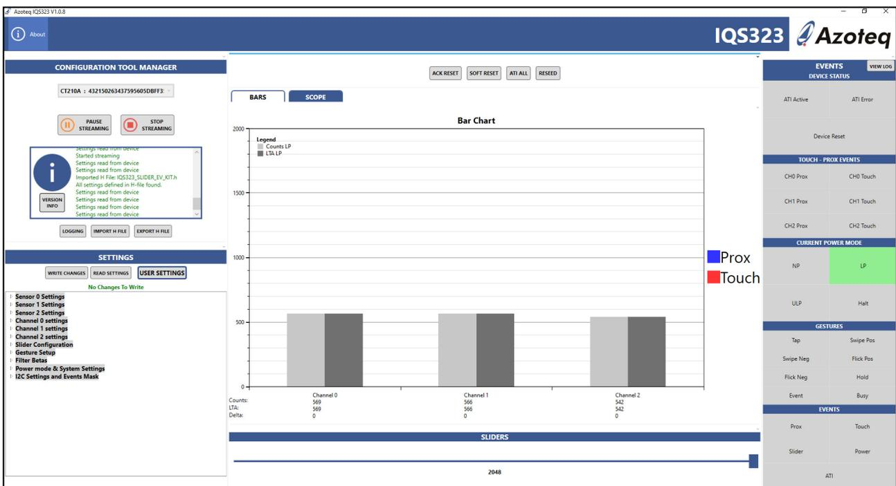
Channel 0 represents the left of the slider. Channel 1 represents the middle of the slider. Channel 2 represents the right of the slider. The LED will turn on when a touch is made on the slider. The slider bar at the bottom of the GUI shows the relative position of the finger on the slider.
