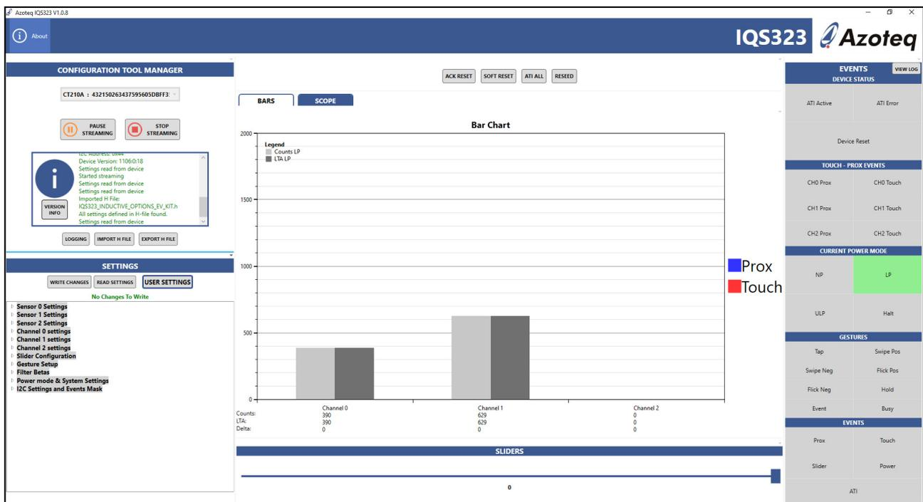
Channel 0 represents the PCB Coil on the left. Channel 1 represents the SMD Coil underneath the metal snap dome on the right. When metal is placed on the PCB Coil, a "Touch" event occurs. The Perspex with attached conductive tape can be used. Press the snap dome above the SMD Coil to observe a "Touch event". The LED will turn on when a "Touch" event is detected.
