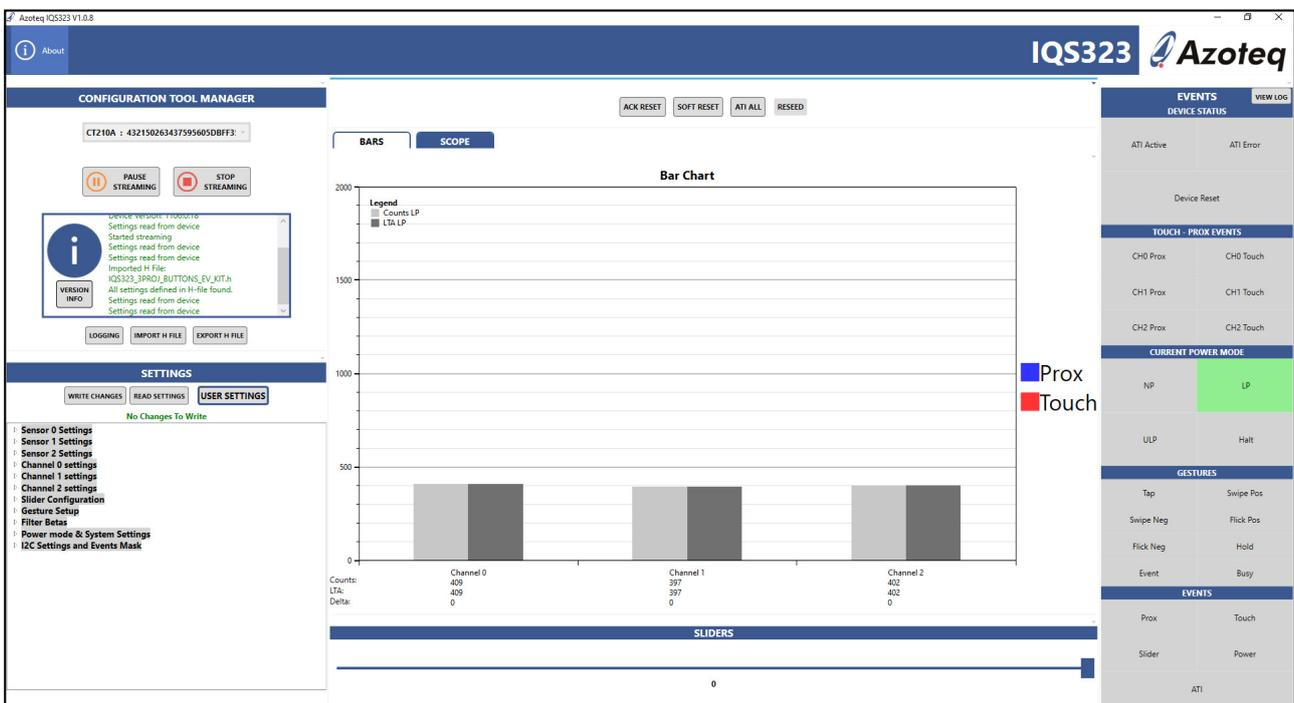
Channel 0 represents Button number 1. Channel 1 represents Button number 2. Channel 2 represents Button number 3. The LED will turn on when any channel has detected a "Touch" event.
