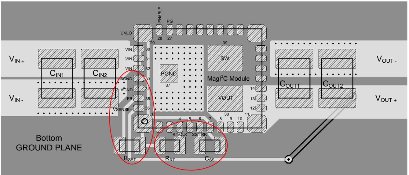
**3: Analog Ground (AGND) to Power Ground (PGND) connections**
