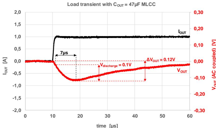
The  $\Delta V_{OUT} = 0.12V$  and  $t_d = 7\mu s$ . It is important to remind that the  $\Delta V_{OUT}$  includes also the voltage drop during  $t_{rise}$ , mainly due to the ESR ( $V_{ESR} = 20mV$ , see picture above). In order to achieve the desired maximum  $\Delta V_{OUT}$ , the  $V_{discharge}$  should be below  $0.06V$ . Using the equation (9), the minimum required output capacitor is:
