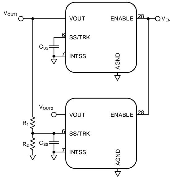
$$R_1 = \frac{V_{OUT2} \cdot 12.6}{V_{REF}} \text{ (k}\Omega\text{)} \quad (10)$$
