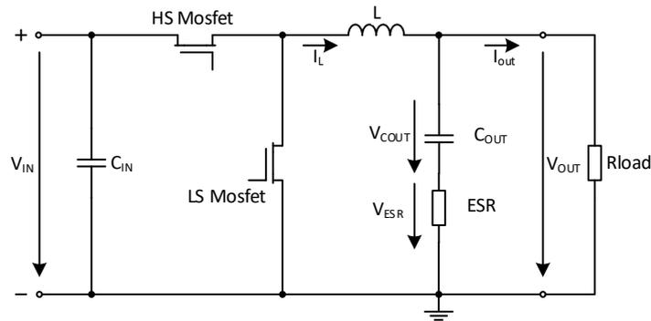
None of the required output capacitors are integrated within the module. The output capacitor must meet the worst case RMS current rating of  $0.5 \cdot \Delta I_L$ , as calculated in equation (4).
