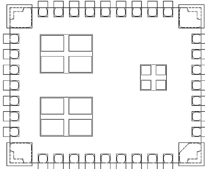
Example solder paste stencil with pins
