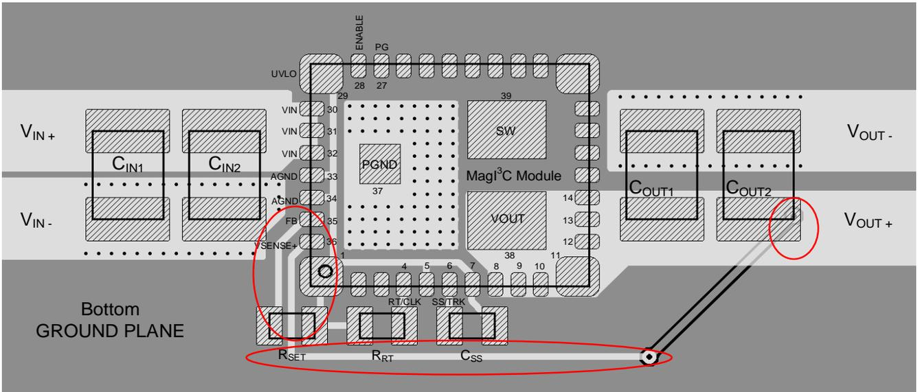
**5: Make input and output bus connections as wide as possible**
