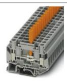
Disconnect terminal block, with knurled screw, for operating the disconnect slide by hand, Connection method: Screw connection, Cross section: 0.5 mm² -10 mm², AWG: 20 - 10, Width: 8.2 mm, Mounting type: NS 35/7,5, NS 35/15, NS 32, Color: gray
