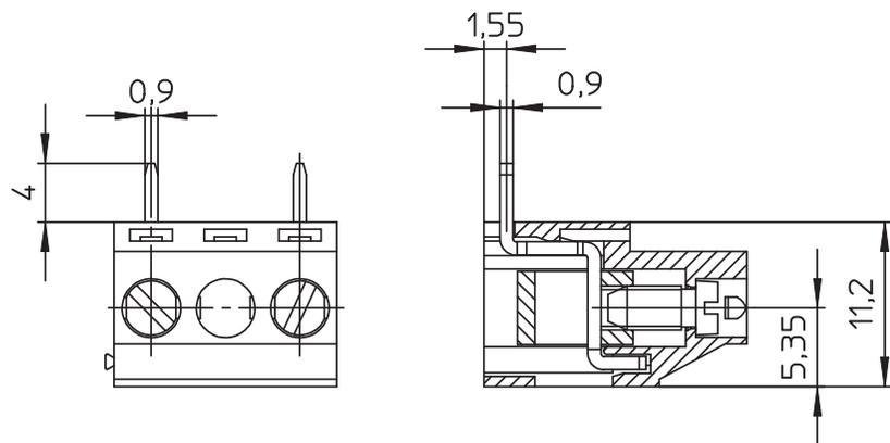
$B = (\text{nb. pin} \times \text{pitch}) - 5,08$
