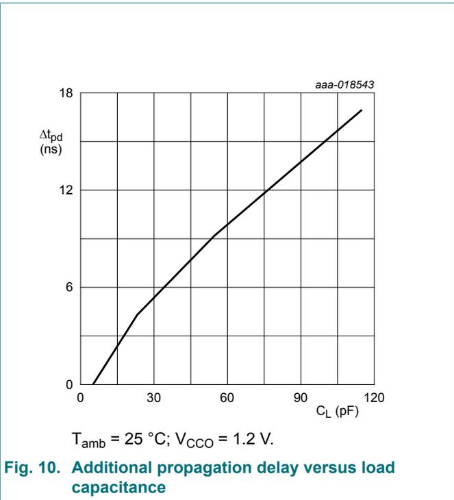
**Fig. 10. Additional propagation delay versus load capacitance**
