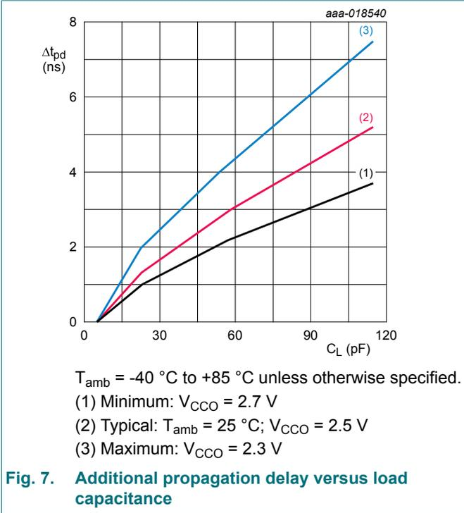
**Fig. 7. Additional propagation delay versus load capacitance**
