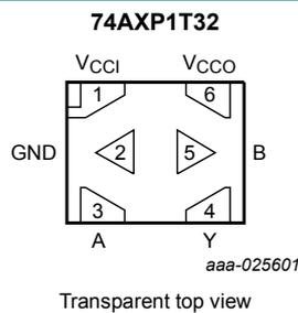
Fig. 3. Pin configuration SOT1255 (X2SON6)
