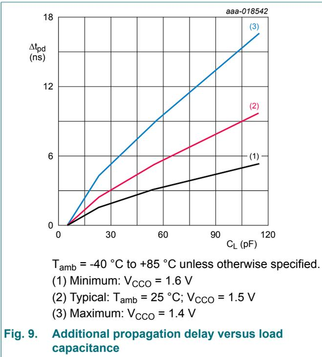
**Fig. 9. Additional propagation delay versus load capacitance**
