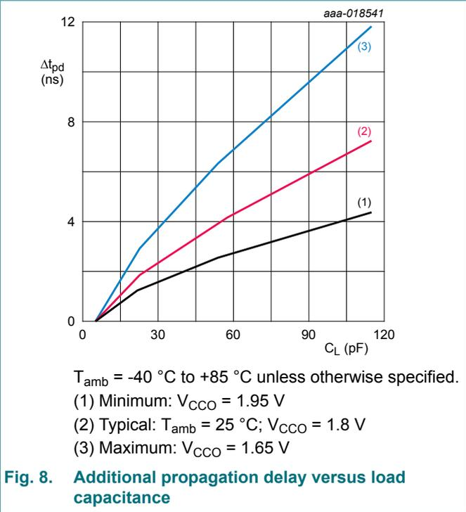
**Fig. 8. Additional propagation delay versus load capacitance**
