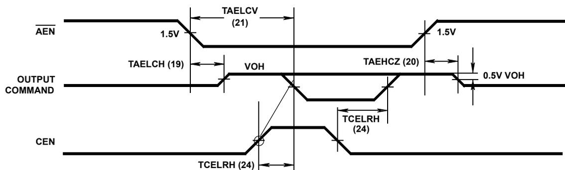
CEN MUST BE LOW OR INVALID PRIOR TO T2 TO PREVENT THE COMMAND FROM BEING GENERATED.
