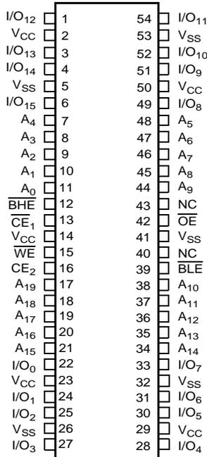
Figure 10. 54-pin TSOP II (22.4 x 11.84 x 1.0 mm) pinout, Dual Chip Enable with ERR, CY7C1061GE<sup>[6, 7]</sup>
