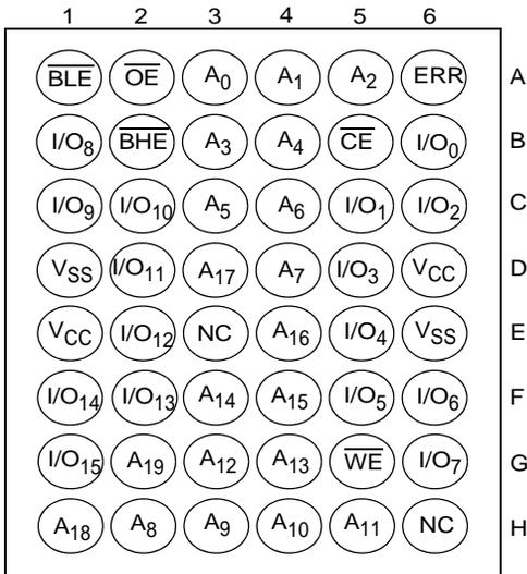
Figure 5. 48-ball VFBGA (6 × 8 × 1.0 mm) Pinout, Dual Chip Enable with ERR, Address MSB A19 at Ball G2, CY7C1061GE<sup>[4, 5]</sup> Package/Grade ID: BVJXI
