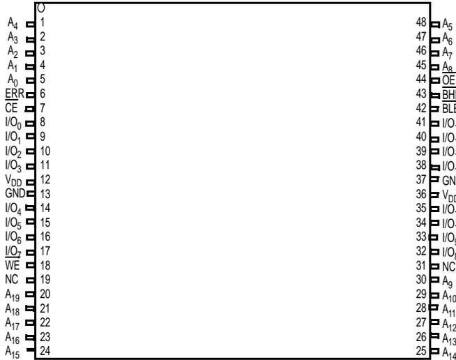
Figure 8. 48-pin TSOP I (12 x 18.4 x 1 mm) Pinout, Single Chip Enable without ERR, CY7C1061G<sup>[6]</sup>
