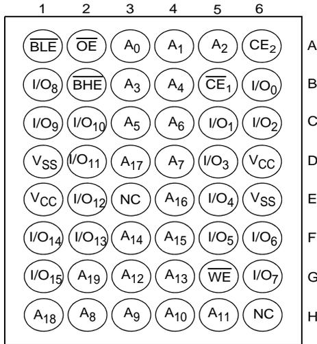
Figure 2. 48-ball VFBGA (6 × 8 × 1.0 mm) Pinout, Dual Chip Enable without ERR, Address MSB A19 at Ball H6, CY7C1061G<sup>[3]</sup> Package/Grade ID: BVXI
