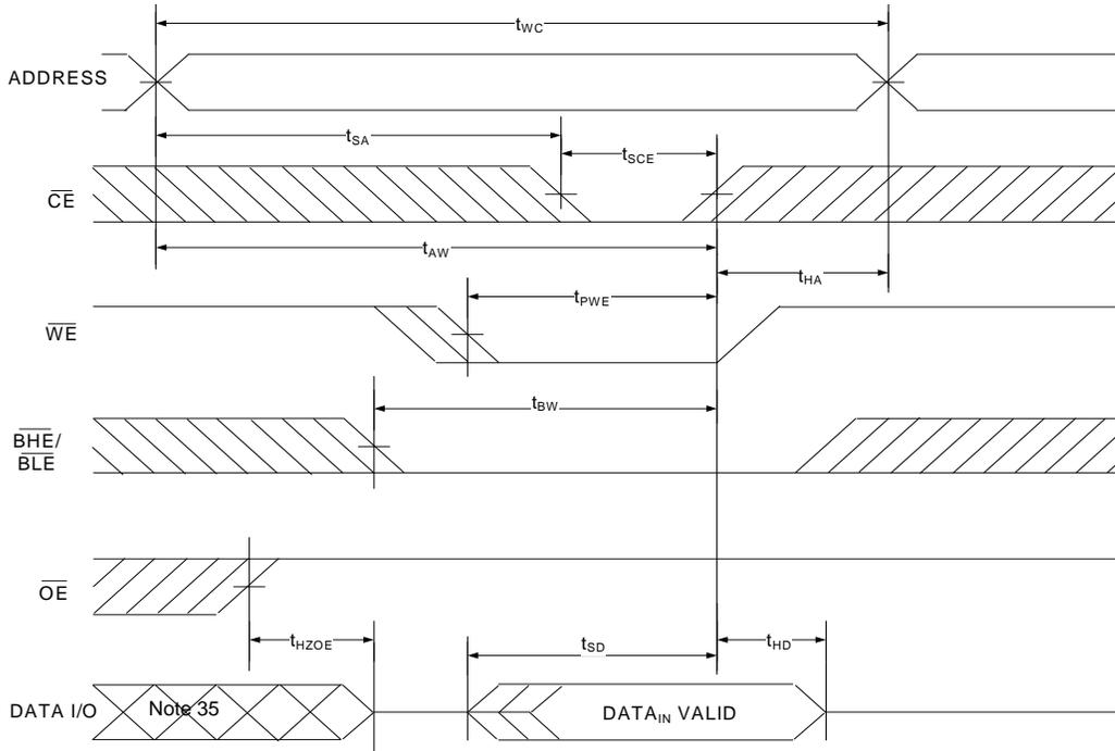
Figure 17. Write Cycle No. 2 ( $\overline{WE}$  Controlled,  $\overline{OE}$  LOW) [31, 32, 33, 34]
