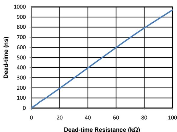
**Figure 37. Dead Time vs. Resistance ( $R_{DT}$ )**
