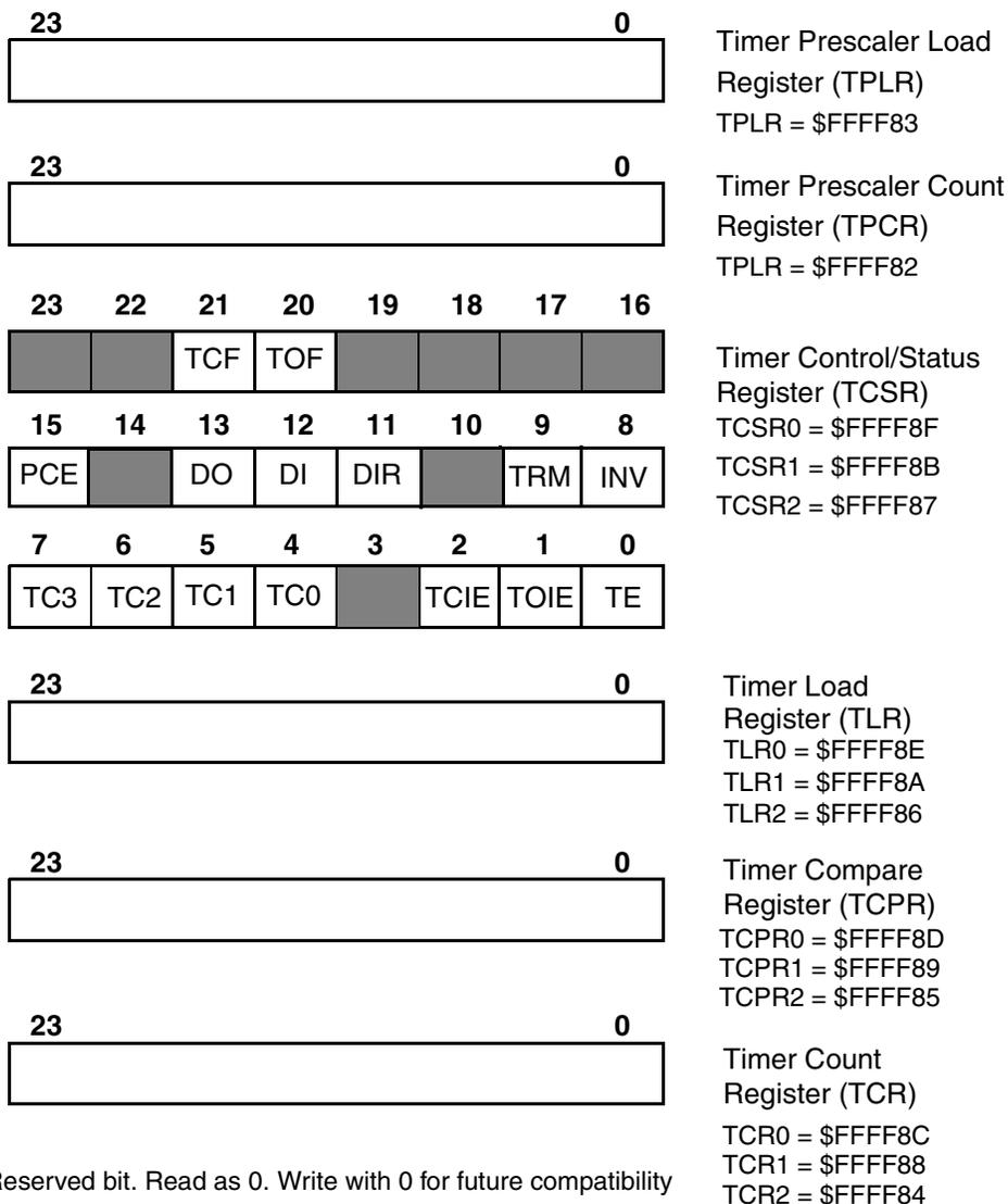
**Figure 9-20.** Timer Module Programming Model
