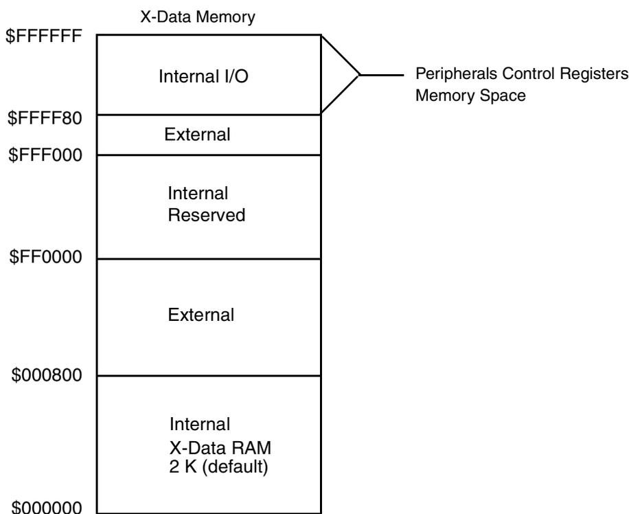
**Figure 5-1.** Memory Mapping of Peripherals Control Registers
