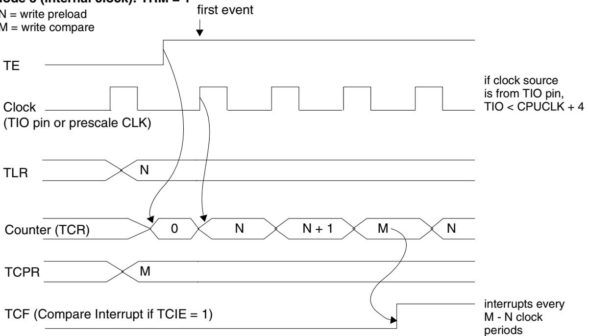
NOTE: If INV = 1, counter is clocked on 1-to-0 clock transitions, instead of 0-to-1 transitions.
