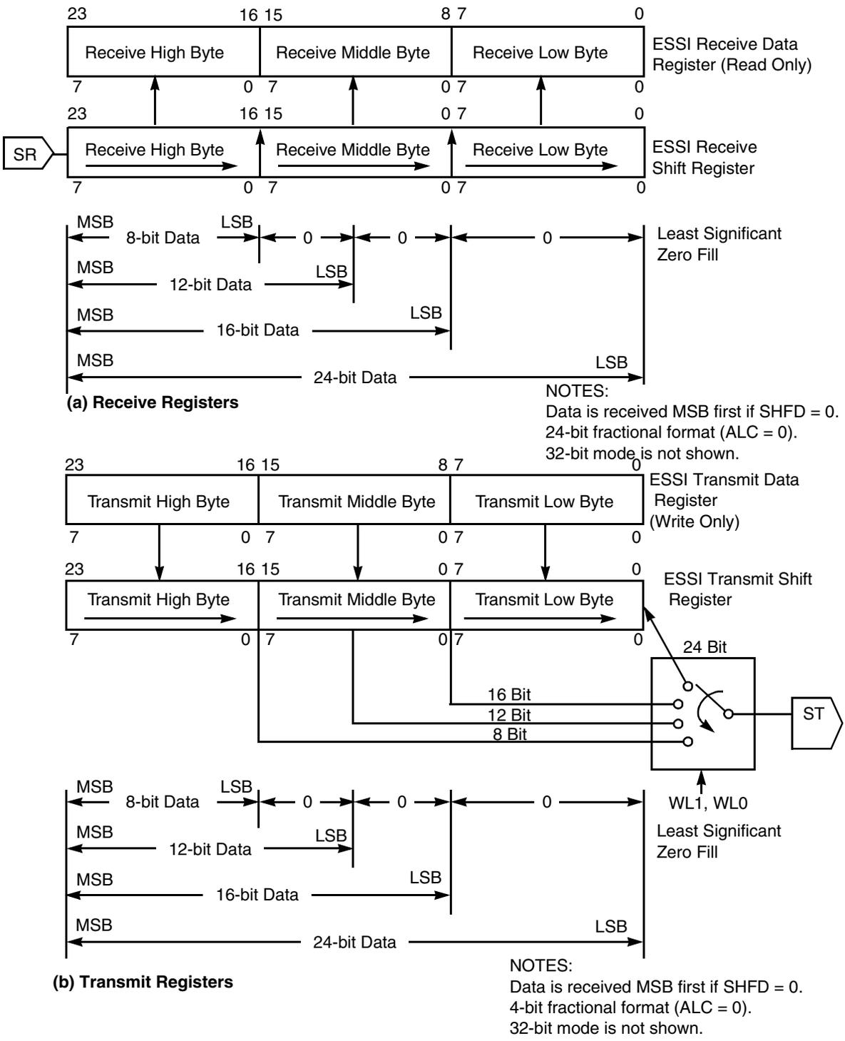
**Figure 7-13. ESSI Data Path Programming Model (SHFD = 1)**
