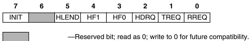
**Figure 6-15. Interface Control Register (ICR)**
