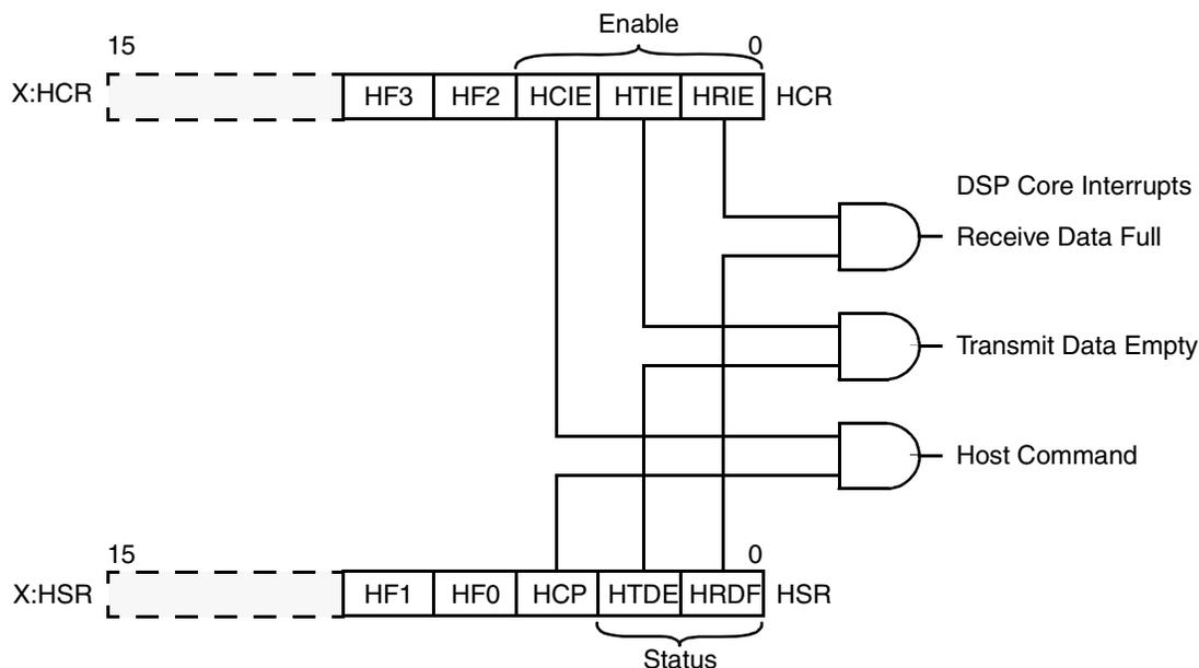
**Figure 6-2.** HI08 Core Interrupt Operation
