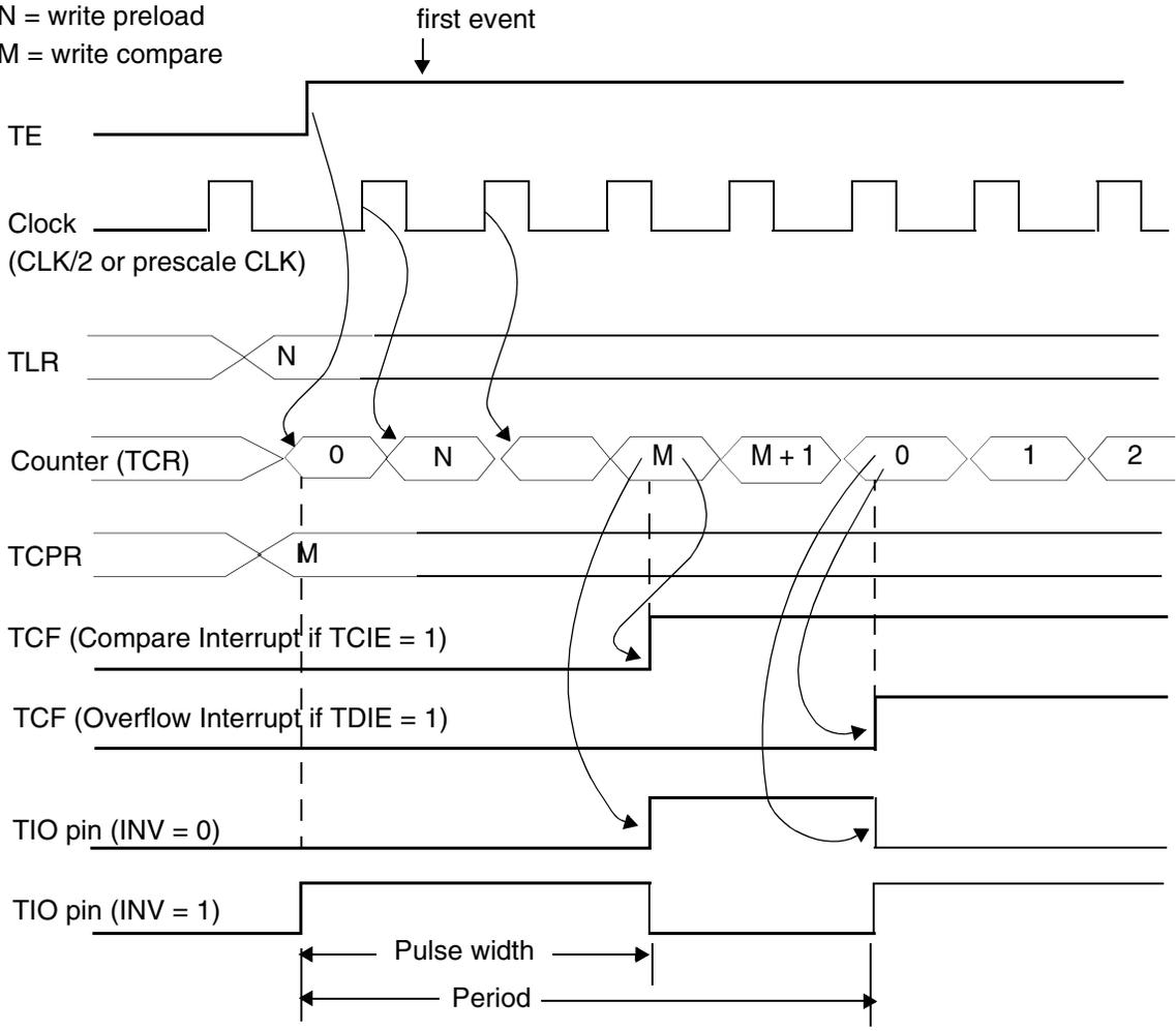
NOTE: On overflow, TCR is loaded with the value of TLR.
