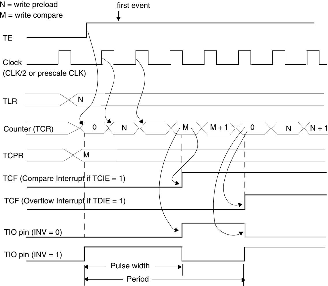
**Figure 9-16.** Pulse Width Modulation Toggle Mode, TRM = 1
