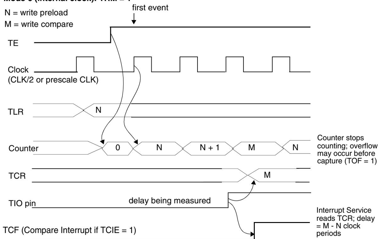
NOTE: If INV = 1, a 1-to-0 edge on TIO loads TCR with count and stops the counter.
