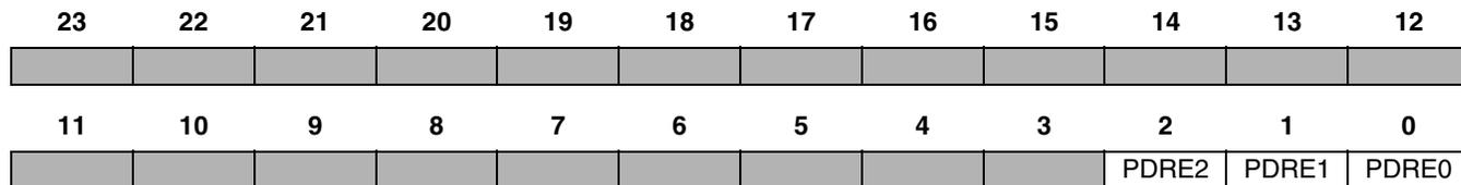
**Note:** For bits 2–0, the value represents the level that is written to or read from the associated signal line if enabled as a GPIO signal by the PCRE bits. For SCI, the GPIO signals are PE[2–0]. The corresponding data bits are PDRE[2–0].
