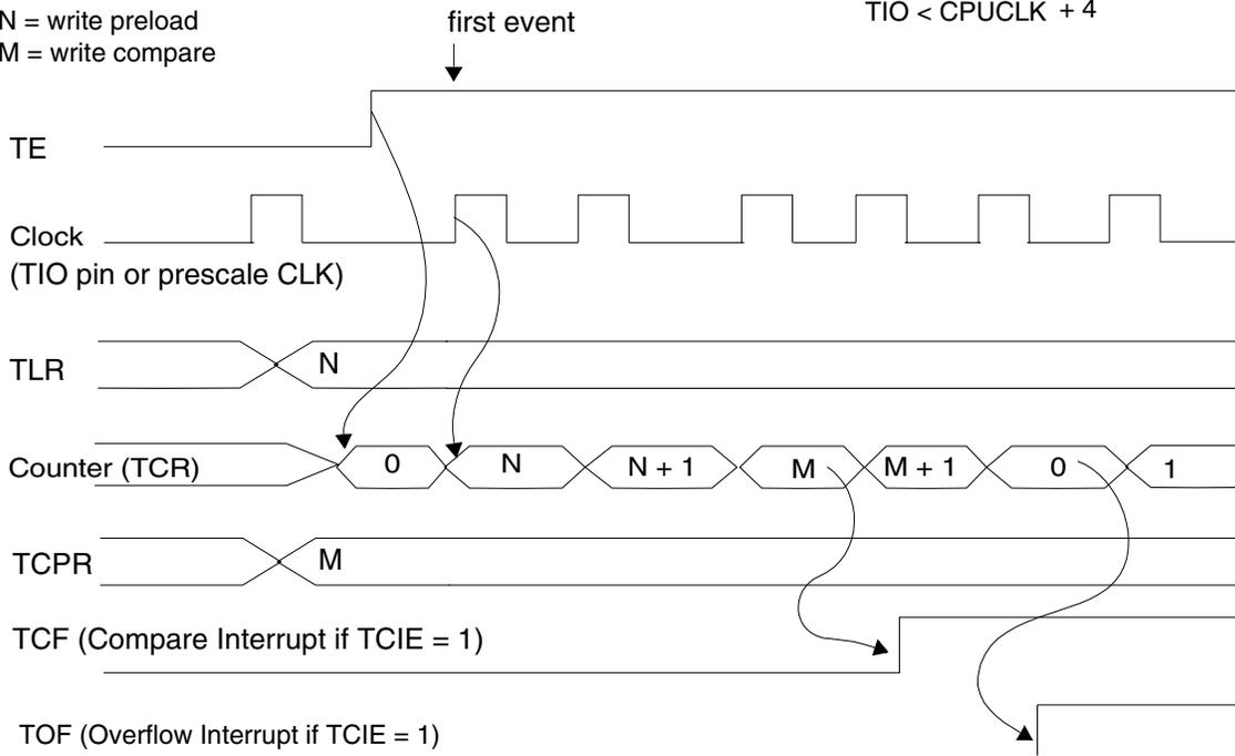
NOTE: If INV = 1, counter is clocked on 1-to-0 clock transitions, instead of 0-to-1 transitions.
