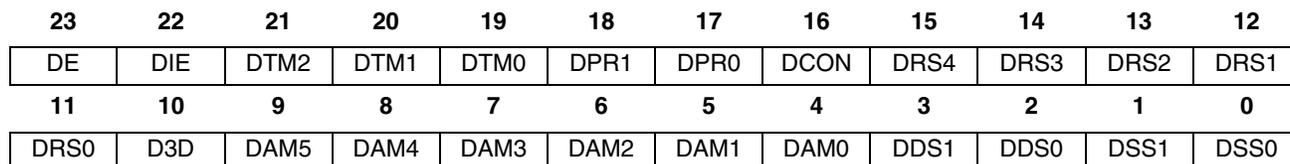
**Figure 4-9. DMA Control Register (DCR)**
