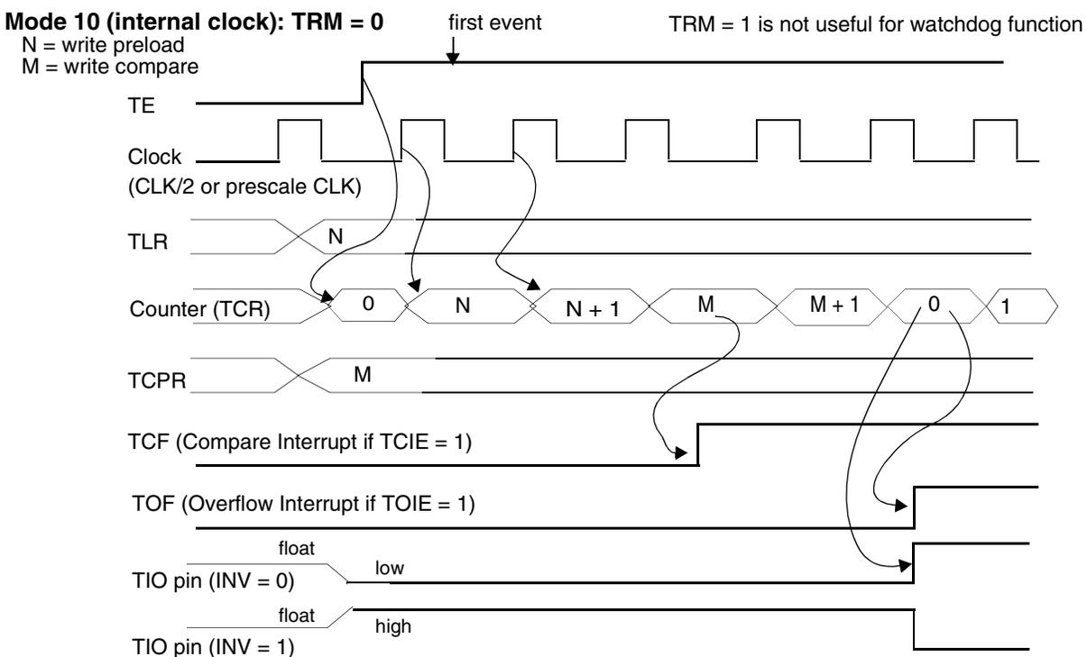
TIO can connect to the RESET pin, internal hardware preserves the TIO value and direction for an additional 2.5 clocks to ensure a reset of valid length.
