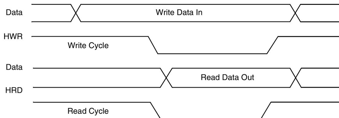
In dual-strobe mode, separate HRD and HWR signals specify the access as a read or write access, respectively.
