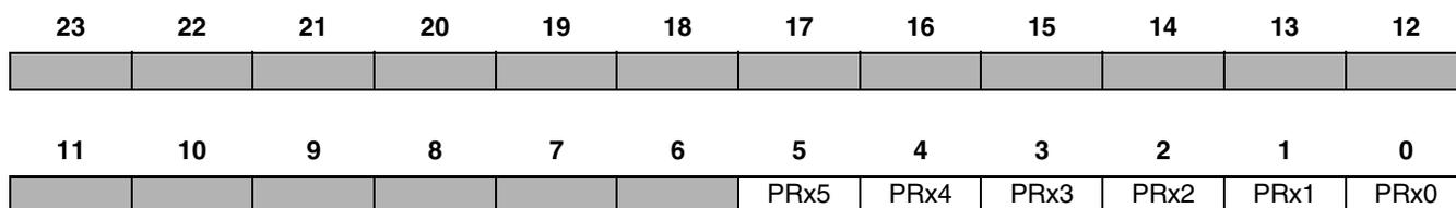
**Note:** For bits 5–0, a 0 configures PR<sub>xn</sub> as a GPI and a 1 configures PR<sub>xn</sub> as a GPO. For ESSI0, the GPIO signals are PC[5–0]. For ESSI1, the GPIO signals are PD[5–0]. The corresponding direction bits for Port C GPIOs are PRC[5–0]. The corresponding direction bits for Port D GPIOs are PRD[5–0].
