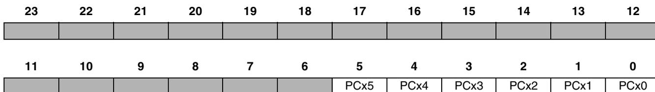
**Note:** For P<sub>x</sub>[5–0], a 0 selects P<sub>xn</sub> as the signal and a 1 selects the specified ESSI signal. For ESSI0, the GPIO signals are PC[5–0] and the ESSI signals are STD0, SRD0, SCK0, and SC0[2–0]. For ESSI1, the GPIO signals are PD[5–0] and the ESSI signals are STD1, SRD1, SCK1, and SC1[2–0].
