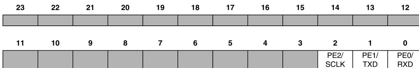
**Note:** For bits 2–0, a 0 selects PEn as the signal and a 1 selects the specified SCI signal.
