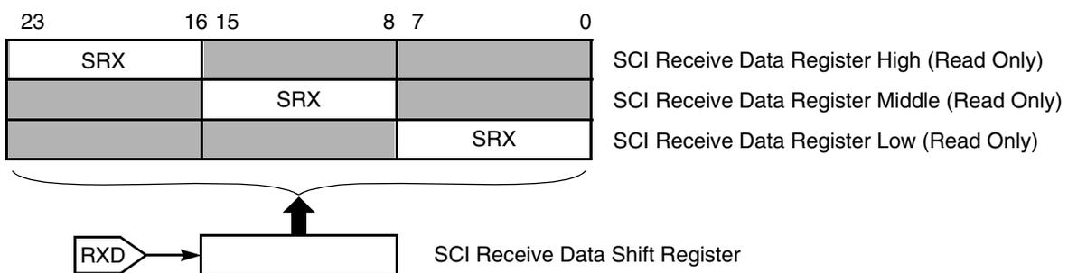
Note: SRX is the same register decoded at three different addresses.
