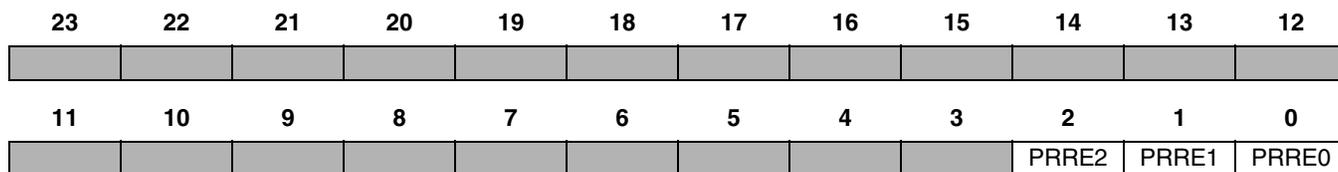
**Note:** For bits 2–0, a 0 configures PE<sub>n</sub> as a GPI and a 1 configures PE<sub>n</sub> as a GPO. For the SCI, the GPIO signals are PE[2–0]. The corresponding direction bits for Port E GPIOs are PRRE[2–0].
