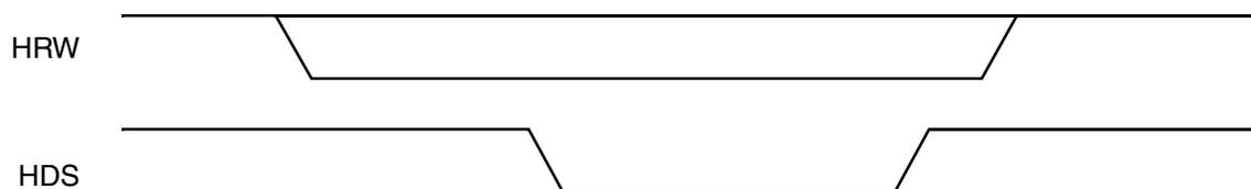
In a single-strobe mode, a DS (data strobe) signal qualifies the access, while a R/W (Read-Write) signal specifies the direction of the access.
