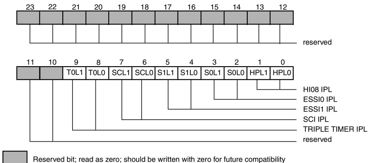
**Figure 4-4.** Interrupt Priority Register-Peripherals (IPRP) (X:\$FFFFFFE)
