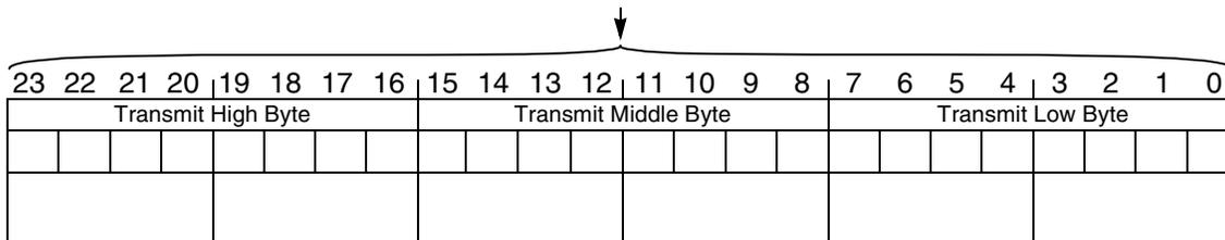
**Host Transmit Data Register (HTX) X:\$FFFC7 Write Only**
