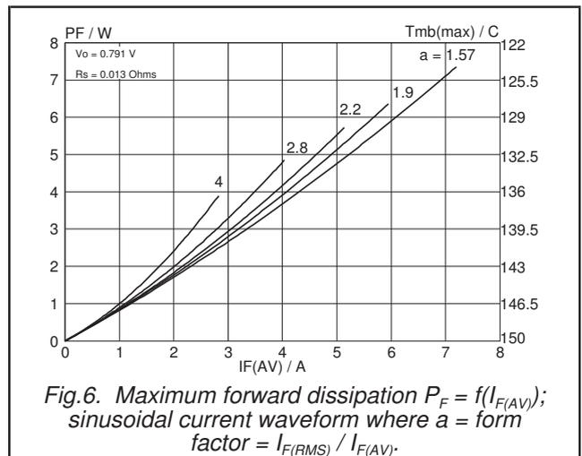
Fig.6. Maximum forward dissipation  $P_F = f(I_{F(AV)})$ ; sinusoidal current waveform where  $a = \text{form factor} = I_{F(RMS)} / I_{F(AV)}$ .
