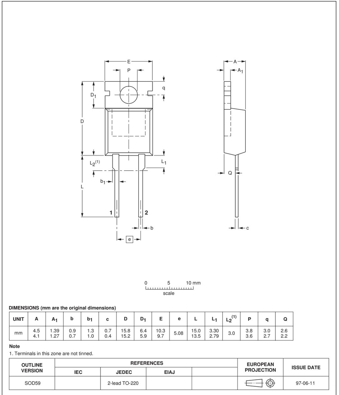
Fig.12. TO220AC; pin 1 connected to mounting base.
