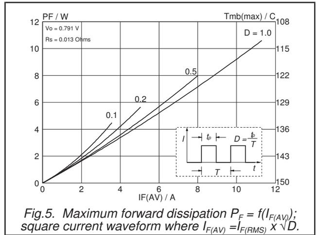
Fig.5. Maximum forward dissipation  $P_F = f(I_{F(AV)})$ ; square current waveform where  $I_{F(AV)} = I_{F(RMS)} \times \sqrt{D}$ .
