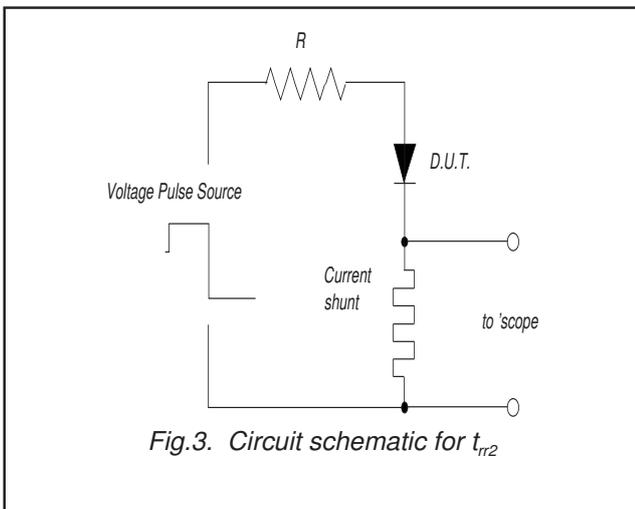
Fig.3. Circuit schematic for  $t_{rr2}$
