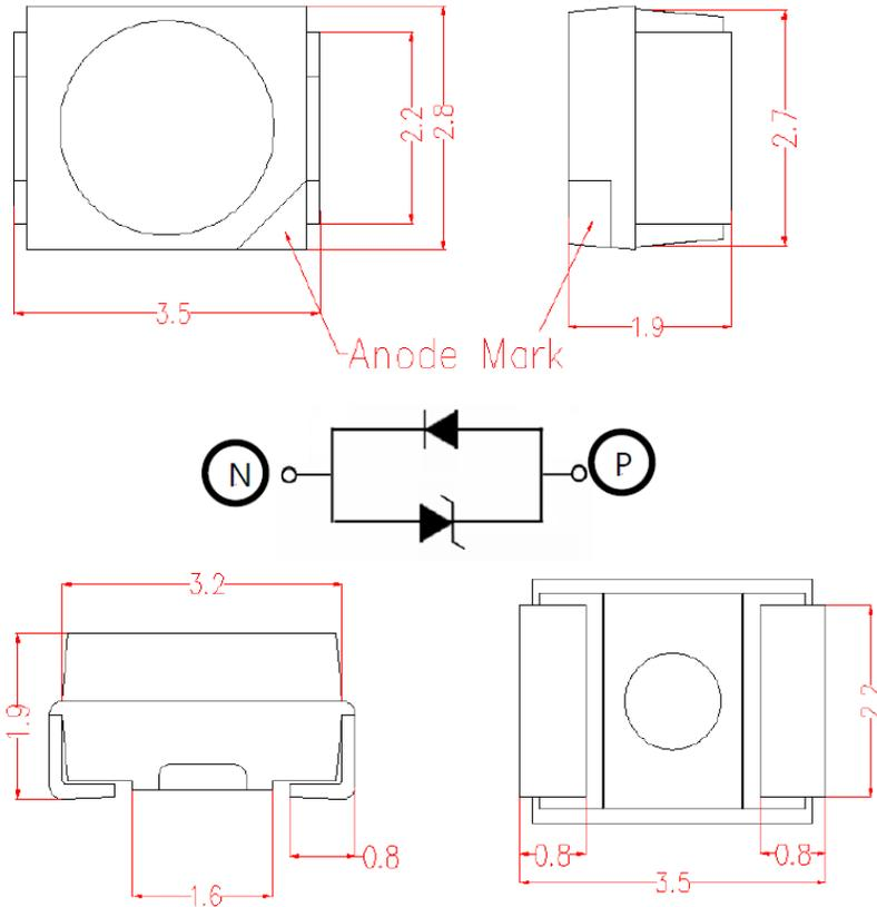
\* All dimensions are in millimeters, \* Tolerances are  $\pm 0.10\text{mm}$ .
