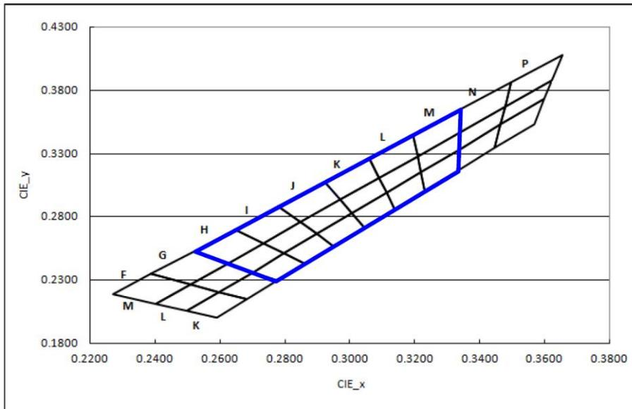
Tolerance of measurements of the Chromaticity Coordinate is  $\pm 0.005$ .
