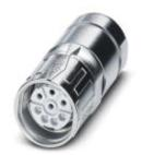
Cable connector, straight short, SPEEDCON locking, M23, number of positions: 5+PE, type of contact: Socket, Crimp connection, shielded: yes, cable diameter range: 9 mm ... 11 mm
