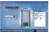
Open the family bootloader V1.0 GUI using the path "Start>Programs>Freescale>JS Family Bootloader." The USB bootloader GUI is shown above.
