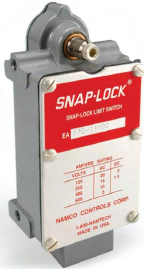
Double pole, double break, double throw, heavy duty limit switch having mechanical travel of 10° to trip and with two normally open and two normally closed circuit.
