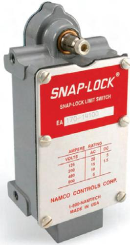
This heavy duty limit switch operates with two normally open and two normally closed circuits, with mechanical travel of less than 6½° required to trip.
