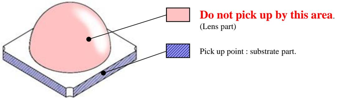
13. Low hardness resin is used for lens. Please avoid overload to the surface of lens which might cause chip-outs, encapsulant delamination, and deformation, nicks, wire disconnection and decreasing reliability.
