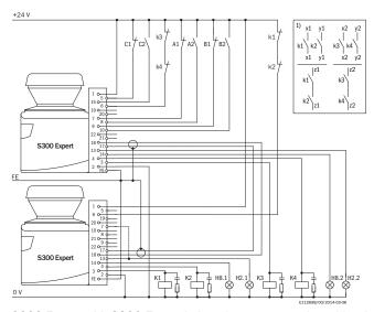
S300 Expert with S300 Expert in host/guest connection with relays/contactors Operating mode: with external device monitoring and without restart interlock Static protective field switching using the control inputs A, B and C The protective fields affect the related OSSDs on host or guest
