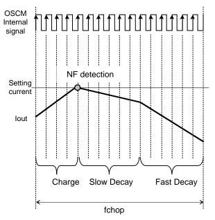
If the NF is detected during the early timing of the fchop cycle, the Slow Decay will be longer.
