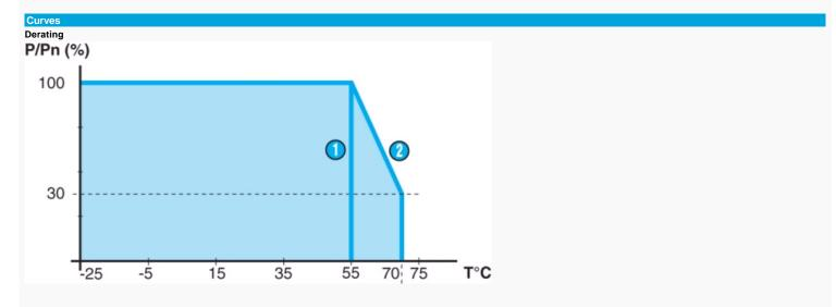
The ambient operating temperature of the Millenium power supplies is 55 °C. Above this, a derating is needed upto a maximum operating temperature of 70 °C. The chart below shows the power (compared to the nominal power) that can be permanently supplied by the power supply, depending on the operating temperature.
