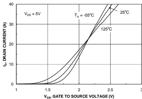
Figure 5. Transfer Characteristics.
