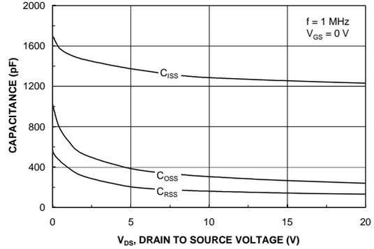
Figure 8. Capacitance Characteristics.
