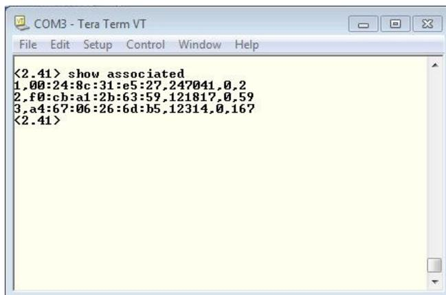
6. View List of Connected Devices using the **show associated** command.
