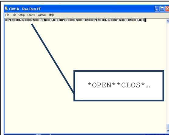
16. Configure the module open a TCP Connection Every 10 seconds, Drops Connection after 3 seconds Inactivity
