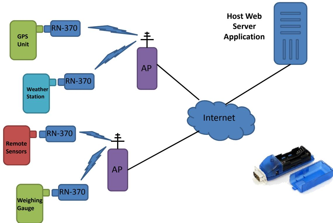
HTTP mode allows you to analog sensor data and module data to a web server as key/value pairs. To enable this mode, use the **set ip proto 18** command. The module connects to a web server using the IP address or URL. The web server listens on port 80 (default) for incoming connections. For each request:
