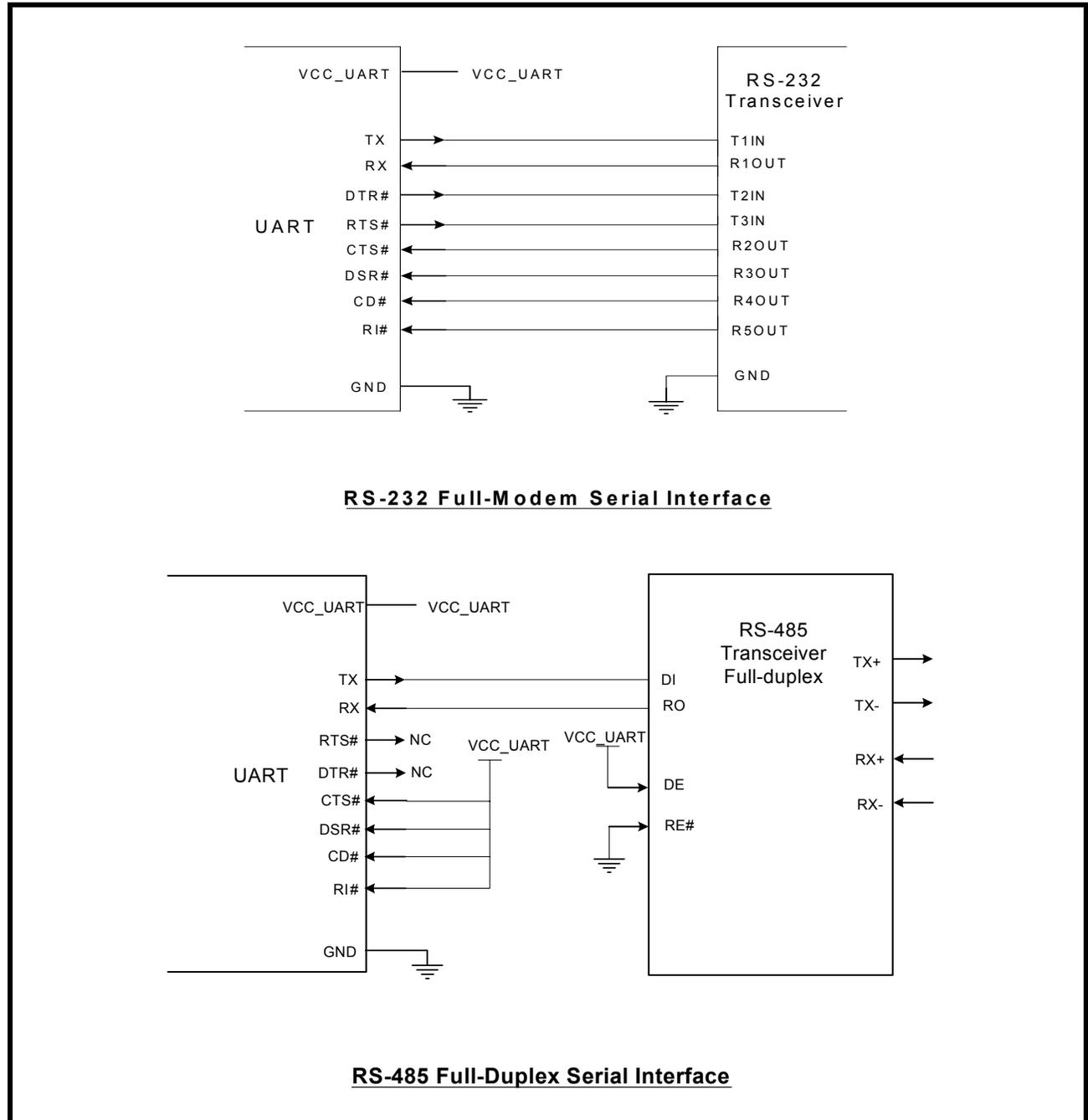
FIGURE 11. XR20M1280 TYPICAL SERIAL INTERFACE CONNECTIONS
