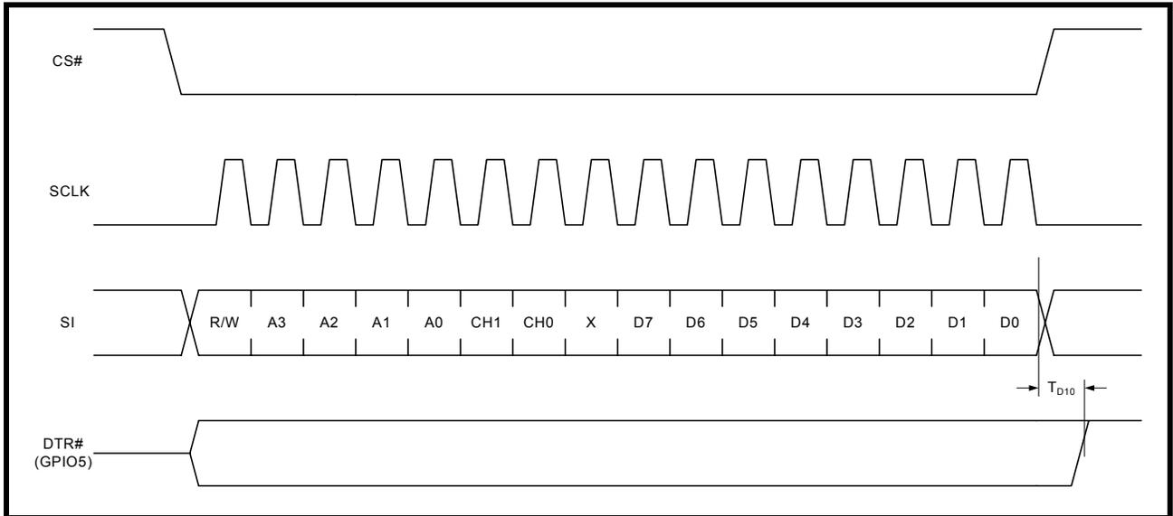
FIGURE 32. SPI WRITE THR TO CLEAR TX INT
