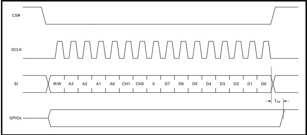
FIGURE 31. SPI WRITE MCR TO DTR OUTPUT SWITCH
