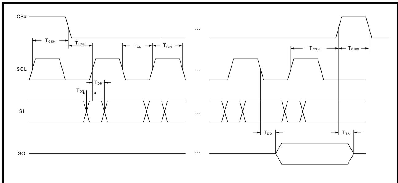
FIGURE 30. SPI WRITE MCR TO DTR OUTPUT SWITCH
