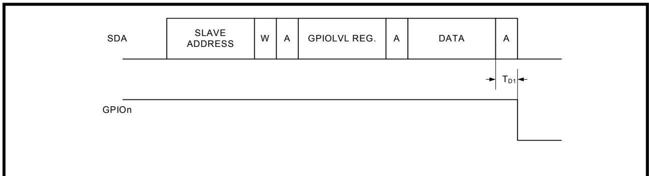
FIGURE 24. MODEM INPUT PIN INTERRUPT
