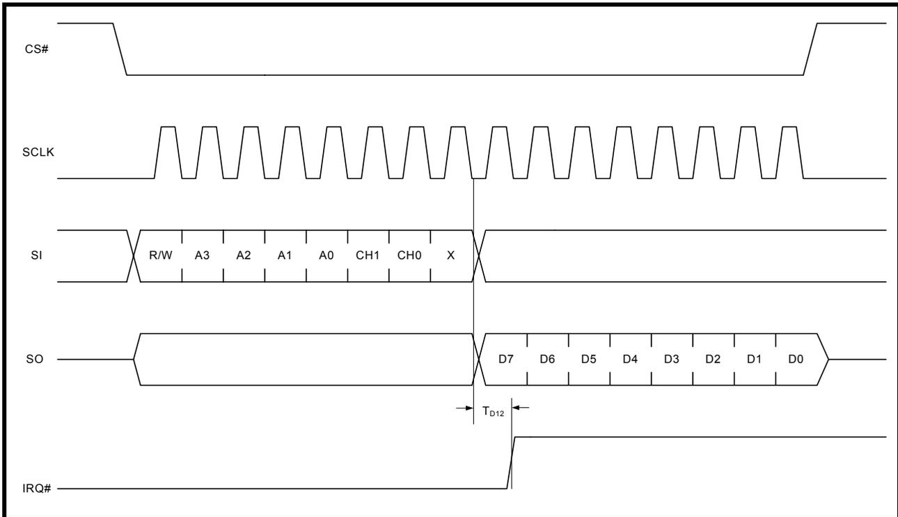
FIGURE 34. READ GPIOVLV TO CLEAR GPIO INT
