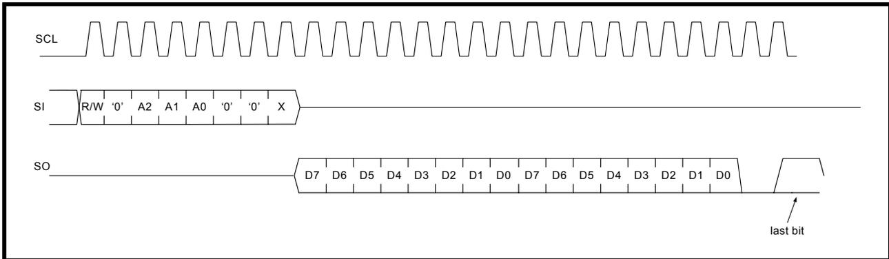
After the last read or write transaction, the SPI master will set the SCL signal back to its idle state (LOW).
