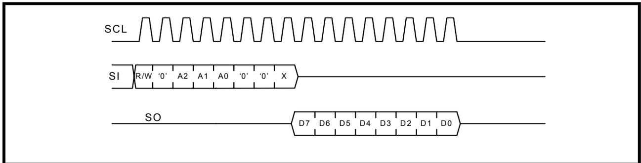
The 128 byte TX FIFO can be loaded with data or 128 byte RX FIFO data can be unloaded in one SPI write or read sequence.
