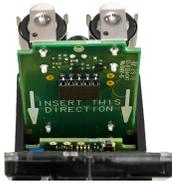
Figure 3: Q45 battery board
