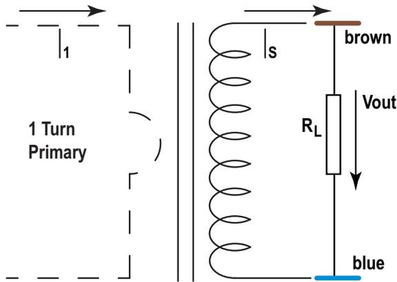
Figure 1: Current transformer wiring
