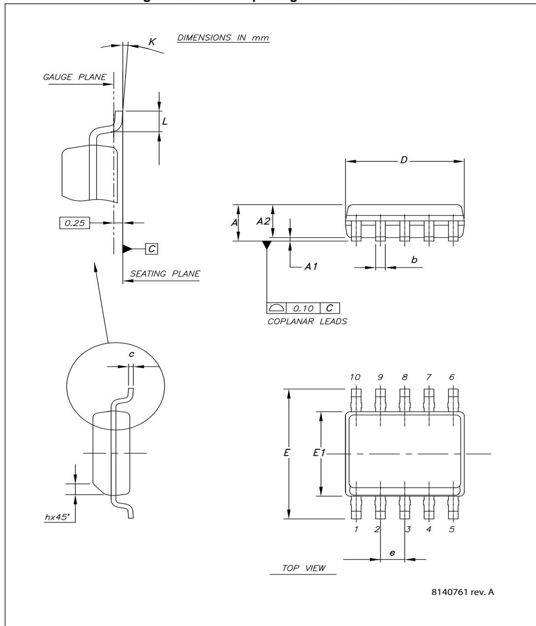
Table 8. SSOP10 package mechanical data
