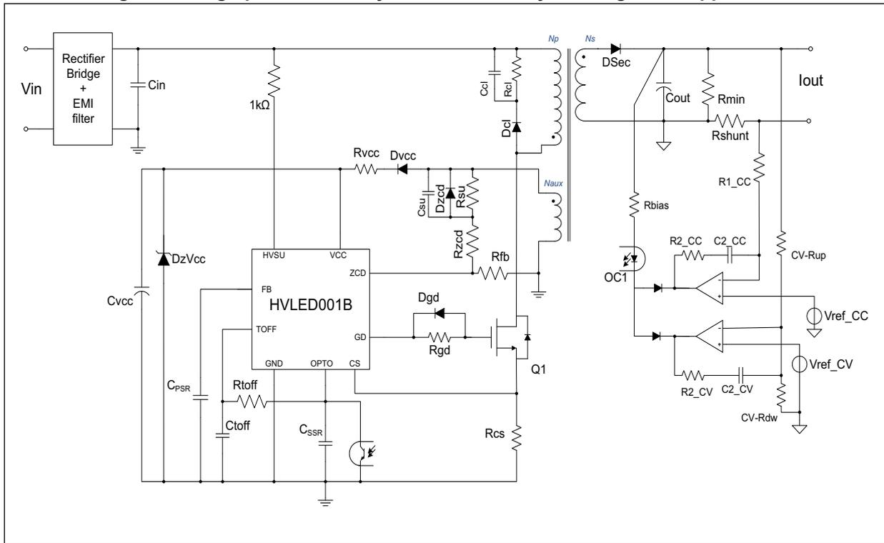
The HVLED001B has five main operating modes: Start-up mode, Ramp-up mode, Active mode, Stop mode and Low consumption mode.
