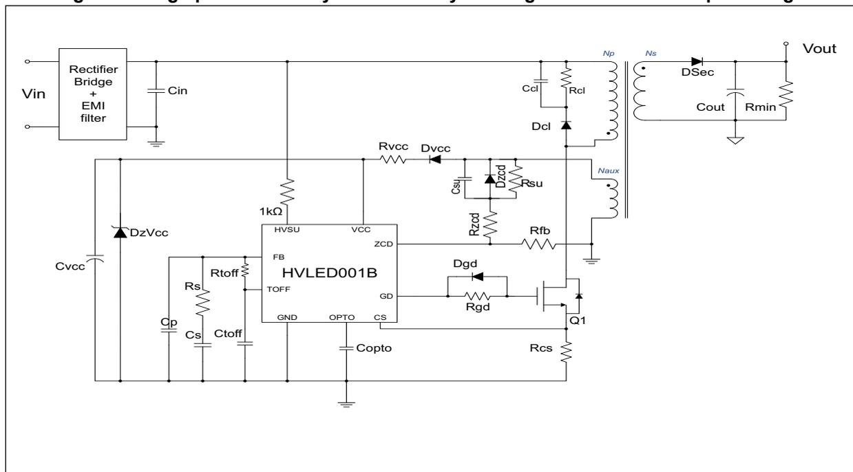
Figure 18. High power factor flyback – secondary side regulated application
