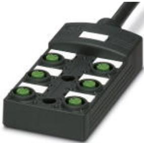
Sensor/actuator box, Connection method: M12-SPEEDCON-socket Plastic, Number of slots: 6, Number of positions: 5, Slot assignment: Double, Status indication: Yes, pnp; Master cable connection: Fixed connection 180°, PUR/PVC, Cable length: 10 m, Shielding: No
