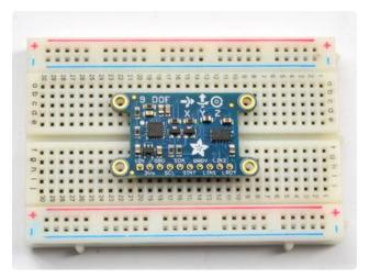
Place the 9DOF board right on top of the header so that the short pins are sticking thru the hole pads
