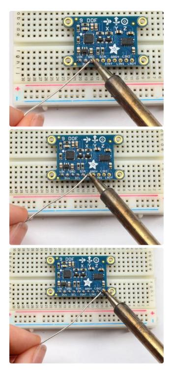
Heat up your soldering iron and once it is ready, solder all 10 pads to the header, making sure to check that there is plenty of solder to make a mechanically strong connection and there's no solder bridging either.
