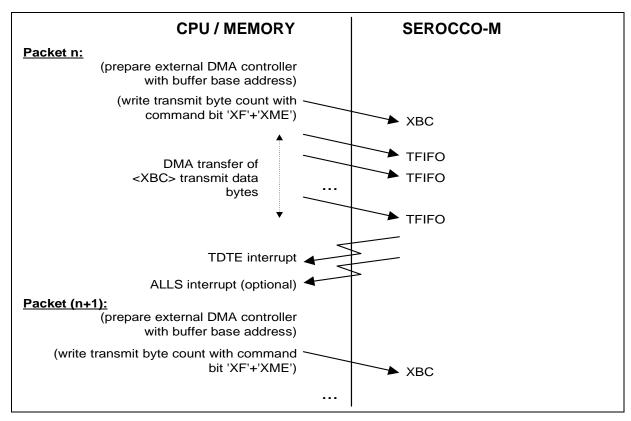
Figure 58 DMA Transmit (Single Buffer per Packet)
