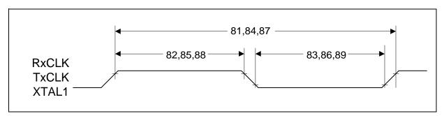
Figure 71 Clock Input Timing
