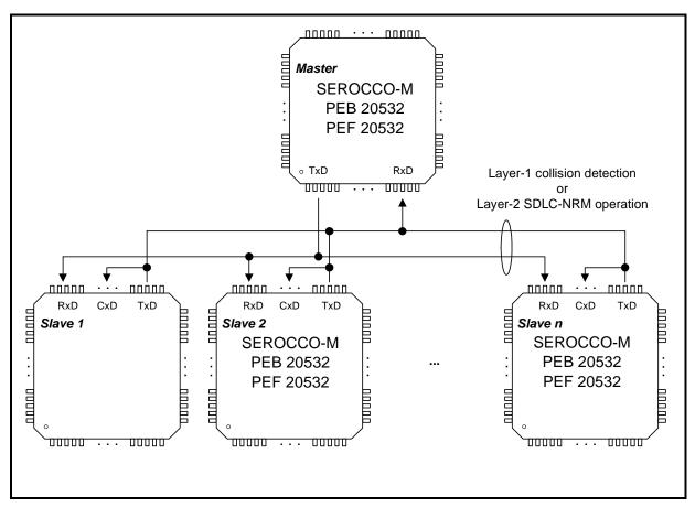
Figure 5 Point-to-Multipoint Bus Configuration
