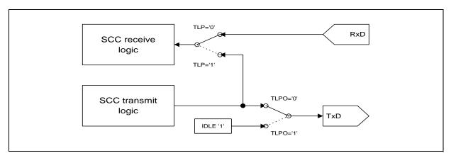
Figure 36 SCC Test Loop
