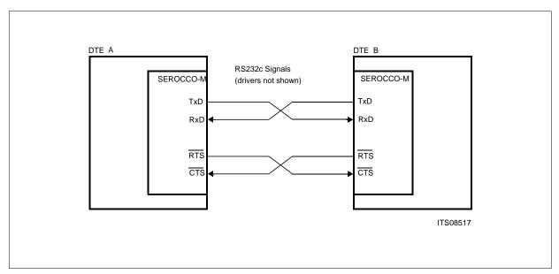
Figure 47 Out-of-Band DTE-DTE Bi-directional Flow Control
