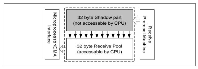
Figure 10 SCC Receive FIFO
