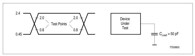
Figure 60 Input/Output Waveform for AC Tests
