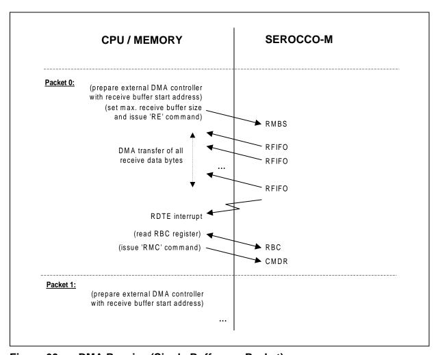
Figure 60 DMA Receive (Single Buffer per Packet)
