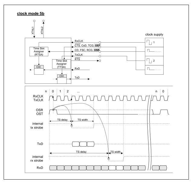
Figure 25 Clock Mode 5b Configuration
