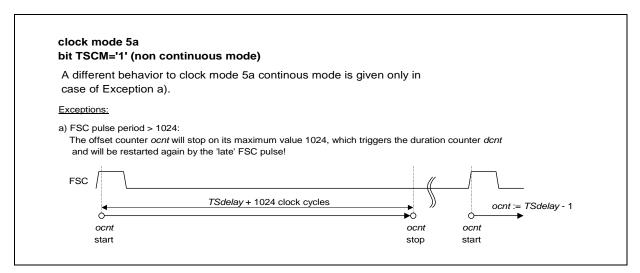
Figure 23 Clock Mode 5a "Non Continuous Mode"
