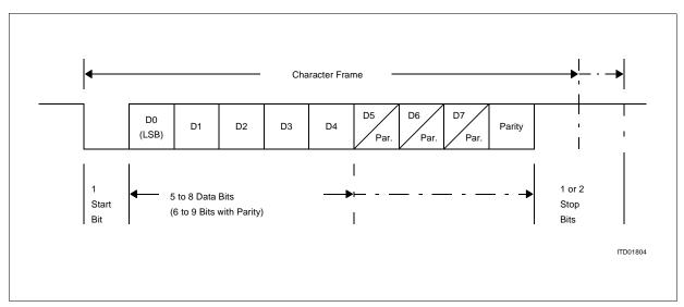
Figure 46 Asynchronous Character Frame
