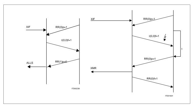
Figure 55 Data Transmission (without error), Data Transmission (with error)
