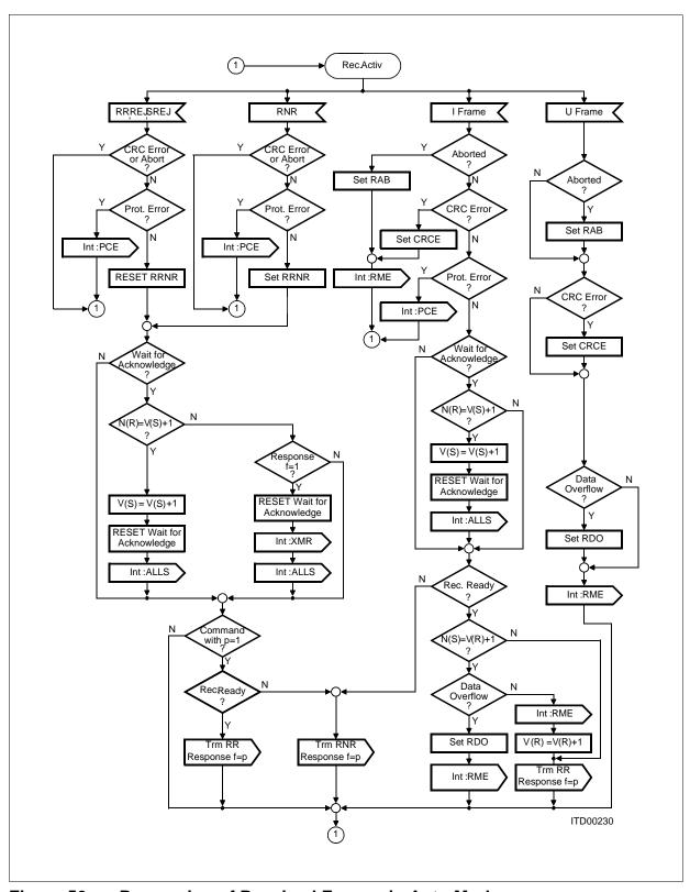
Figure 50 Processing of Received Frames in Auto Mode
