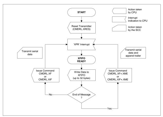
Figure 56 Interrupt Driven Data Transmission (Flow Diagram)
