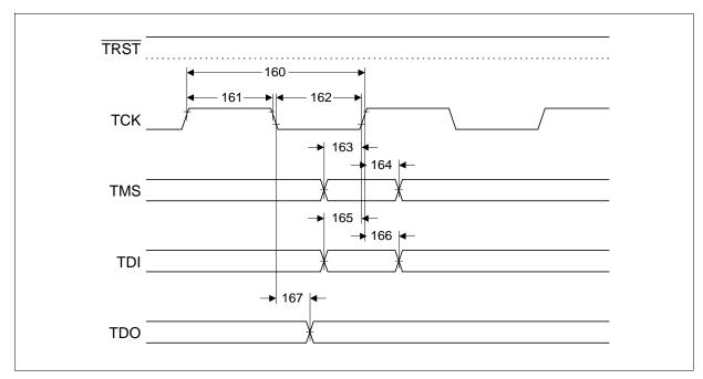
Figure 79 JTAG-Boundary Scan Timing
