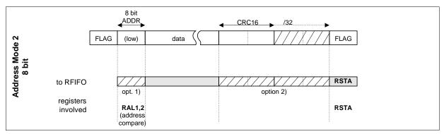
Figure 41 HDLC Receive Data Processing in Address Mode 2 (8 bit)
