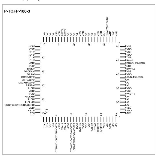
Figure 7 Pin Configuration P-TQFP-100-3 Package
