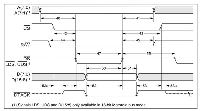
Figure 68 Motorola Write Cycle Timing
