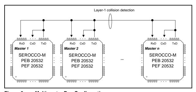
Figure 6 Multimaster Bus Configuration
