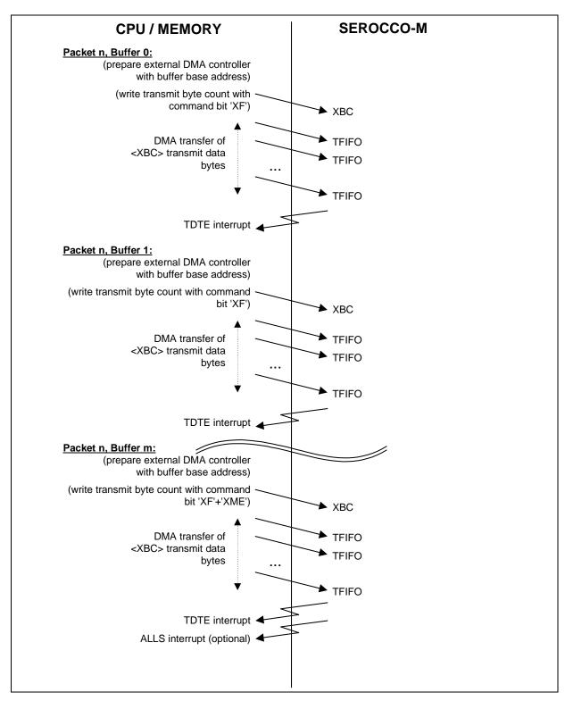
Figure 59 Fragmented DMA Transmission (Multiple Buffers per Packet)
