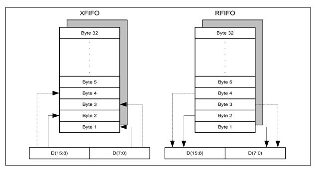
Figure 11 XFIFO/RFIFO Word Access (Intel Mode)
