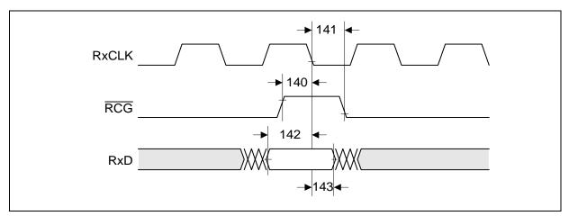
Figure 75 Clock Mode 4 Receive Gating Timing
