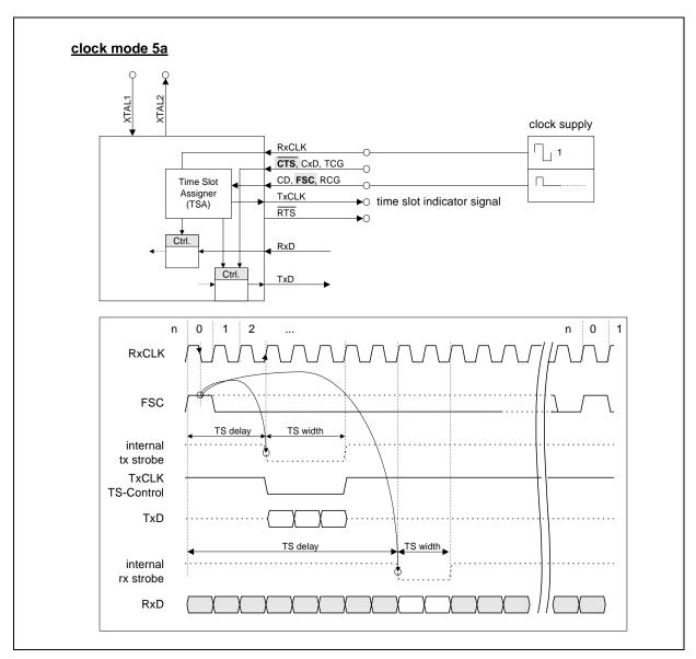
Figure 21 Clock Mode 5a Configuration
