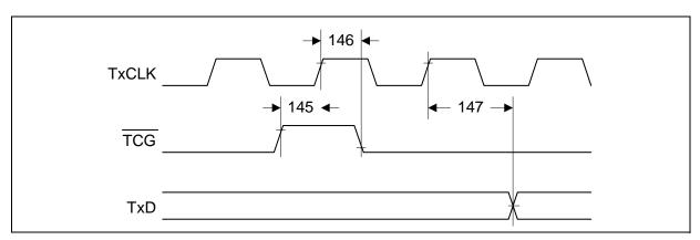
Figure 76 Clock Mode 4 Transmit Gating Timing
