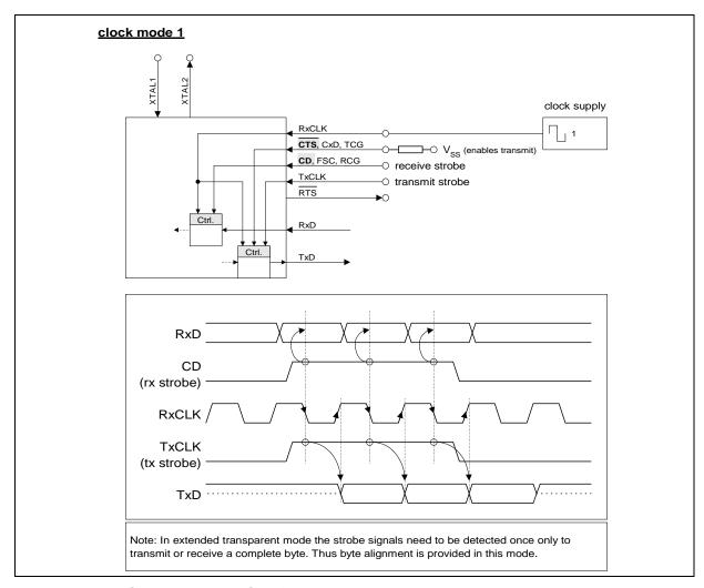
Figure 15 Clock Mode 1 Configuration
