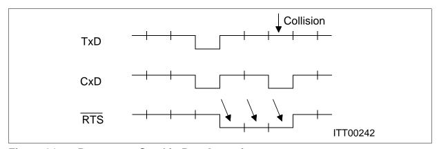
Figure 31 Request-to-Send in Bus Operation
