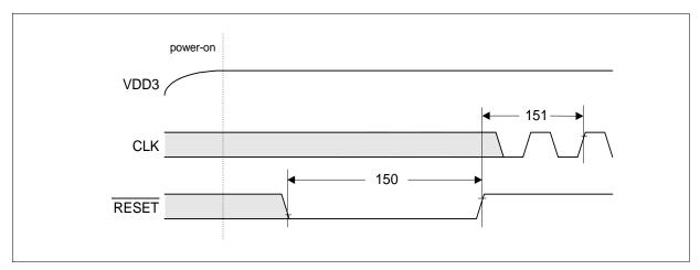
Figure 78 Reset Timing
