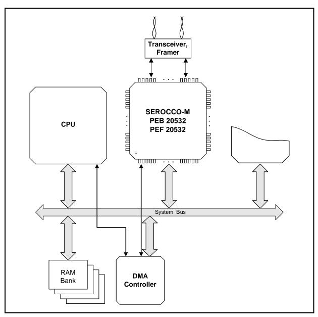
Figure 3 System Integration With External DMA Controller
