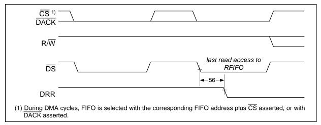
Figure 69 Motorola DMA Read Cycle Timing
