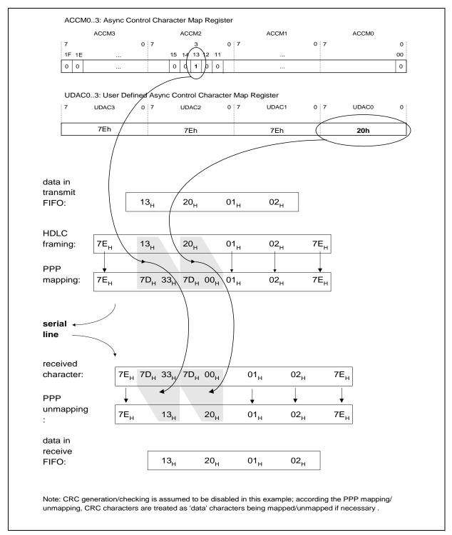
Figure 45 PPP Mapping/Unmapping Example
