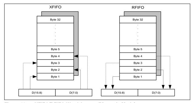
Figure 12 XFIFO/RFIFO Word Access (Motorola Mode)
