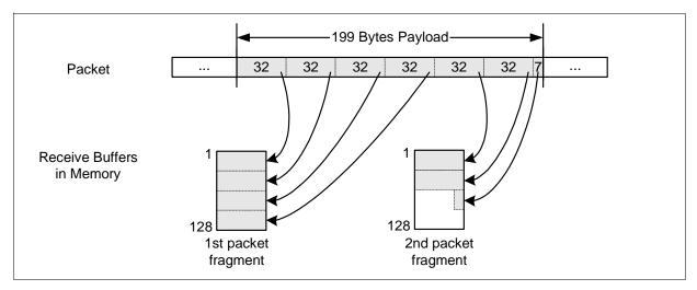
Figure 61 Fragmented Reception per DMA (Example)
