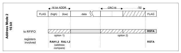
Figure 40 HDLC Receive Data Processing in Address Mode 2 (16 bit)
