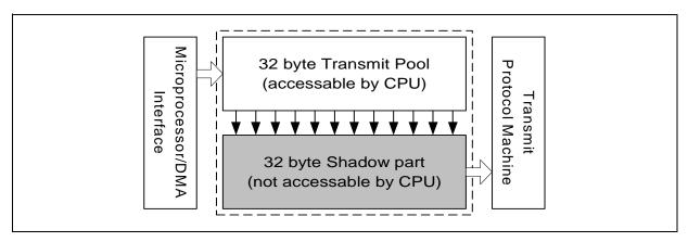
Figure 9 SCC Transmit FIFO
