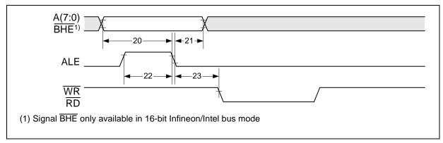
Figure 66 Infineon/Intel Multiplexed Address Timing
