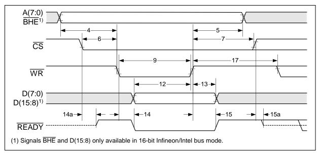
Figure 63 Infineon/Intel Write Cycle Timing
