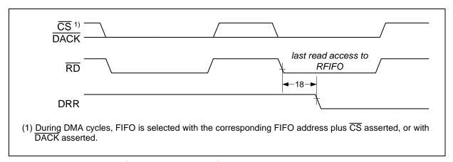
Figure 64 Infineon/Intel DMA Read Cycle Timing
