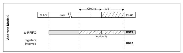
Figure 43 HDLC Receive Data Processing in Address Mode 0
