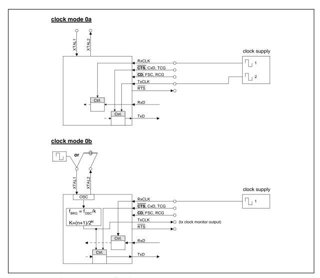
Figure 14 Clock Mode 0a/0b Configuration
