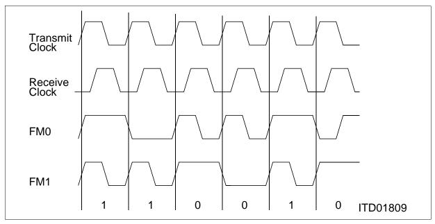
Figure 33 FM0 and FM1 Data Encoding
