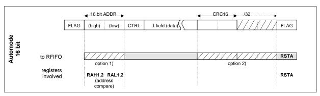
Figure 38 HDLC Receive Data Processing in 16 bit Automode
