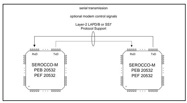
Figure 4 Point-to-Point Configuration
