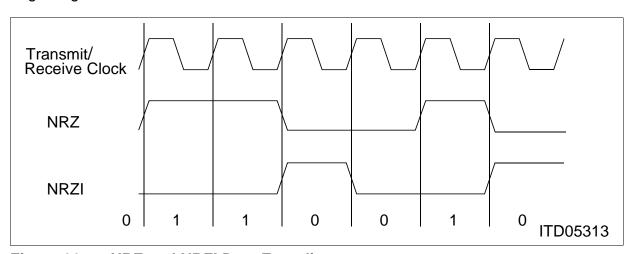
Figure 32 NRZ and NRZI Data Encoding
