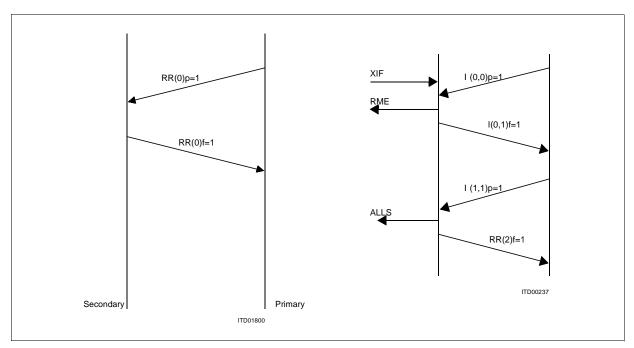
Figure 54 No Data to Send: Data Reception/Transmission
