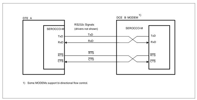
Figure 48 Out-of-Band DTE-DCE Bi-directional Flow Control
