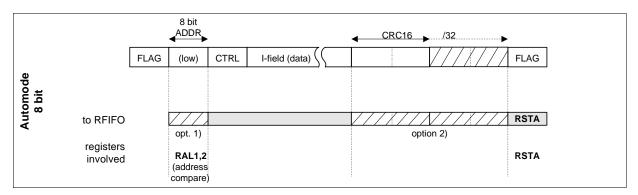
Figure 39 HDLC Receive Data Processing in 8 bit Automode
