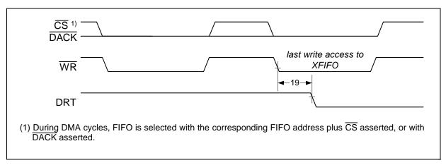
Figure 65 Infineon/Intel DMA Write Cycle Timing
