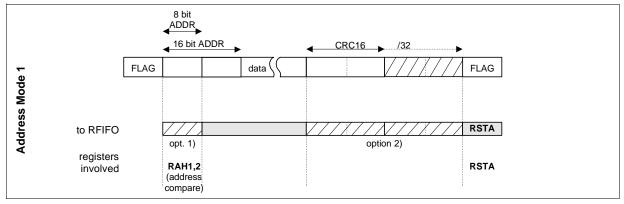
Figure 42 HDLC Receive Data Processing in Address Mode 1
