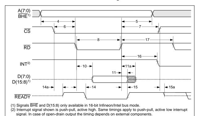
Figure 62 Infineon/Intel Read Cycle Timing
