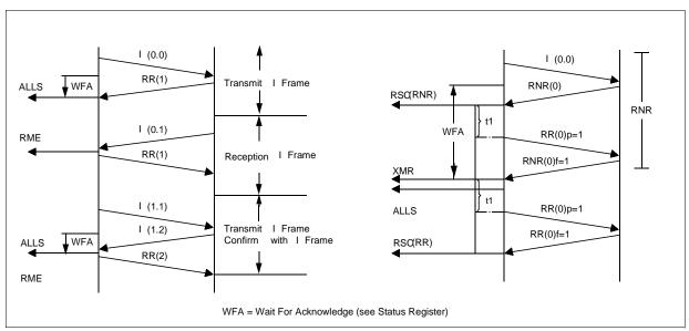
Figure 52 Transmission/Reception of I-Frames and Flow Control
