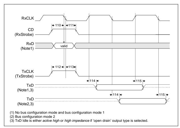
Figure 74 Clock Mode 1 Strobe Timing
