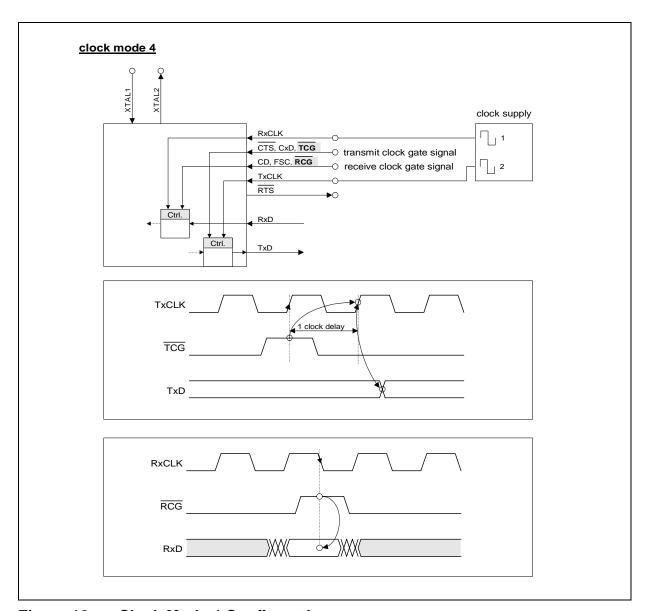
Figure 18 Clock Mode 4 Configuration
