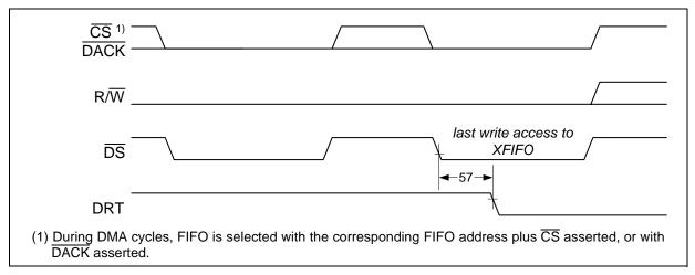
Figure 70 Motorola DMA Write Cycle Timing
