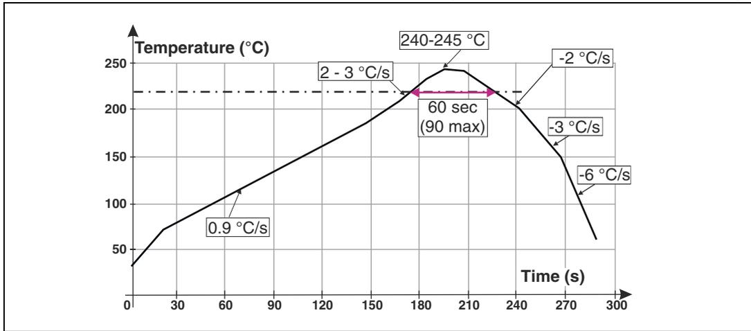
Note: Minimize air convection currents in the reflow oven to avoid component movement.
