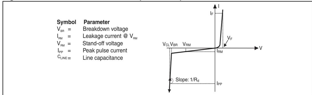
**Table 2. Electrical characteristics ( $T_{amb} = 25^{\circ}C$ )**
