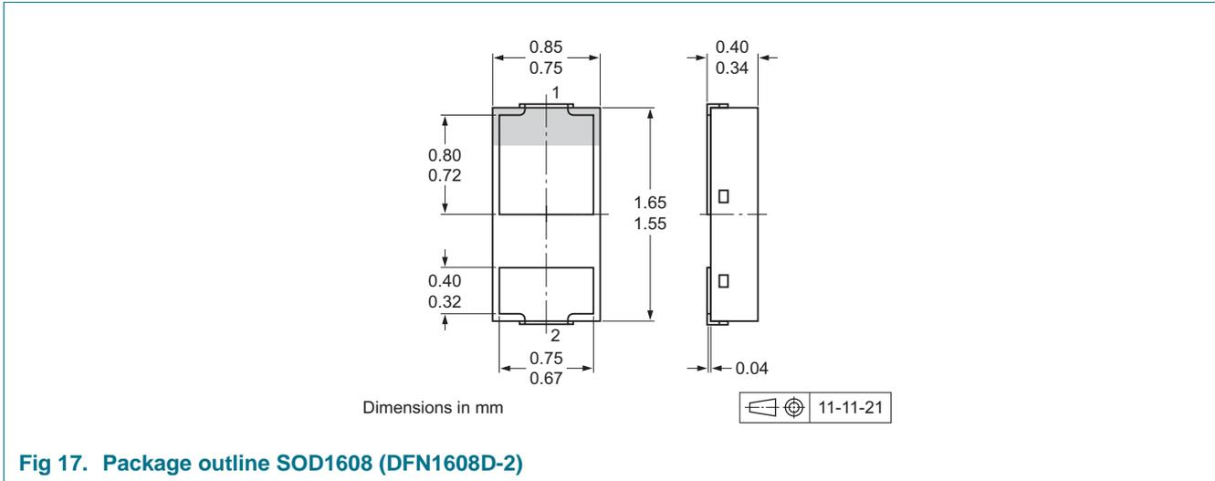
Fig 17. Package outline SOD1608 (DFN1608D-2)
