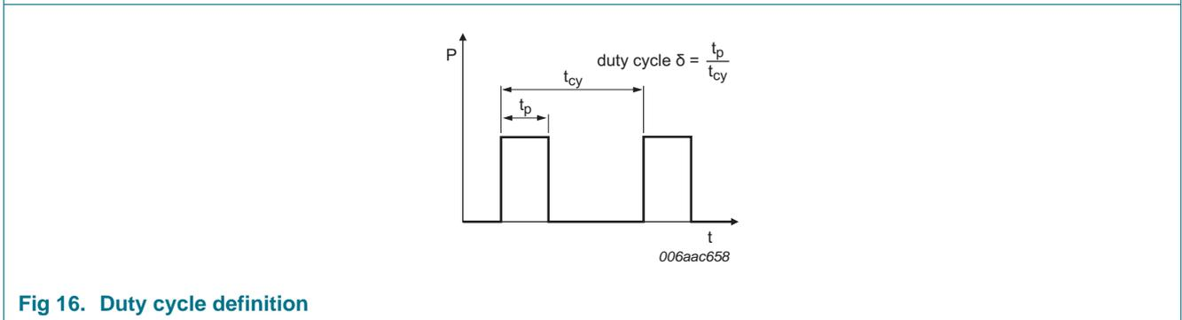
**Fig 16. Duty cycle definition**
