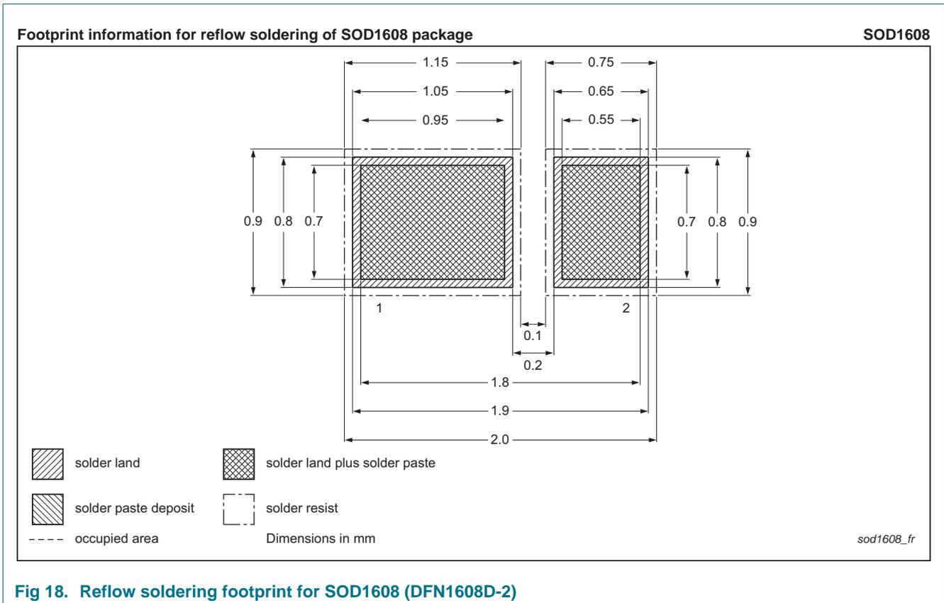
Fig 18. Reflow soldering footprint for SOD1608 (DFN1608D-2)
