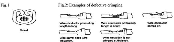
Check of crimping appearance visually for correct crimping as referring to above Fig.2 Check the tensile strength at crimped part when operation finishes.
