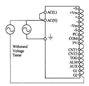
Output ~  $\frac{1}{2}$  (chassis) : 500VAC 1min. (100mA), (SWS600L-60 and SWS1000L-60: 651VAC 1min 130mA)
