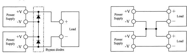
Note : Ensure that all units must be in operation. (Never use in condition that one of the units is not operated.)
