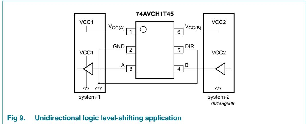
Fig 9. Unidirectional logic level-shifting application
