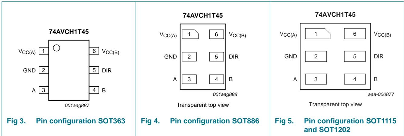
Fig 3. Pin configuration SOT363
