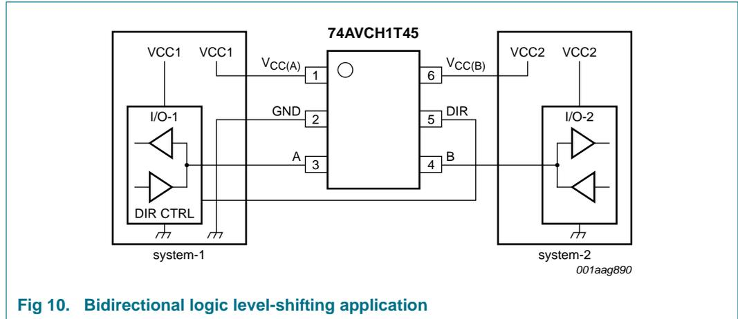
Fig 10. Bidirectional logic level-shifting application
