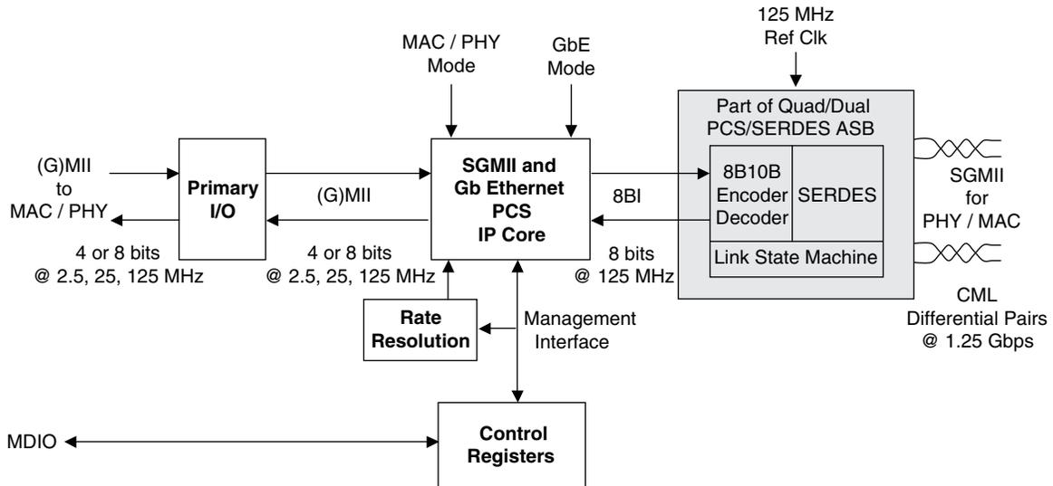
Figure 2-3 shows typical clock network connections between the IP core, the SERDES, and a MAC.
