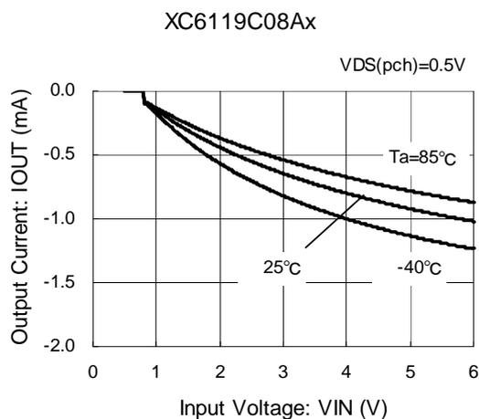
(6) Cd Pin Sink Current vs. Input Voltage
