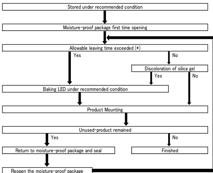
Allowable leaving time means the maximum allowable leaving time after opening package, which depends on each LED type. The allowable leaving time should be calculated from the first opening of package to the time when soldering process is finished. When judging if the allowable leaving time has exceeded or not, please subtract the soldering time. The allowable leaving time after reopening should be calculated from the first opening of package, or from the time when baking process is finished.
