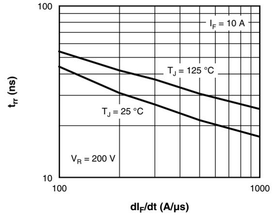
Fig. 7 - Typical Reverse Recovery Time vs.  $di/dt$
