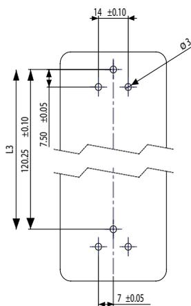
Drilling diagram for PCB terminals: L individua andl N/PE bussed [mm]
