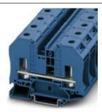
Feed-through terminal block with bolt connection method, cross section: 2.5 - 35 mm², AWG: 14 - 2, width 20.2 mm, color: blue
