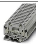
Disconnect terminal block, Connection method: Screw connection, Cross section: 0.5 mm² -10 mm², AWG: 20 - 10, Width: 8.2 mm, Mounting type: NS 35/7,5, NS 35/15, NS 32, Color: gray
