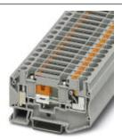
Test disconnect terminal block, With test socket screws for insertion of test plugs, connection method: Pushin connection, Screw connection, cross section: 0.5 mm² - 10 mm², AWG: 20 - 10, width: 8.2 mm, color: gray, mounting: NS 35/7,5, NS 35/15
