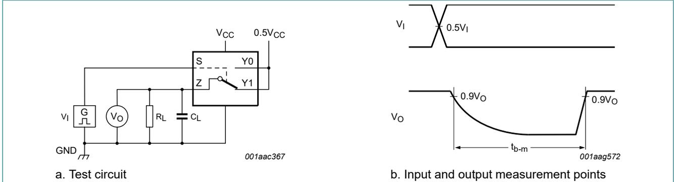
Fig. 14. Test circuit for measuring break-before-make timing
