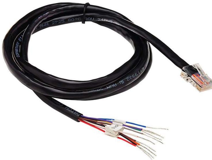
The RJ45/Bare Wire 48" cable provides a customizable connector for connecting EIA422/EIA485 devices to the standard Digi 10 pin RJ45 serial connector. Customers or Integrators can use this cable to make EIA 422/EIA485 connections by attaching the wires to a terminal block or by wiring them into a DB9 or DB25 connector hood for the specific device they wish to use.
