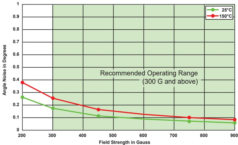
Figure 49: Noise (3 Sigma) over Field Strength
