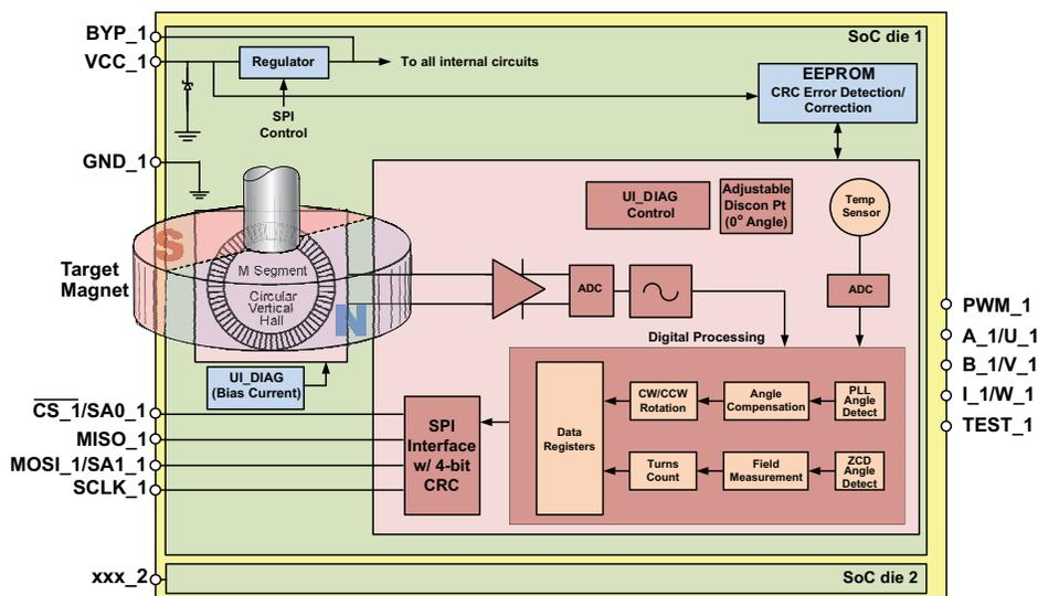
Figure 1: A1333 Magnetic Circuit and IC Diagram
