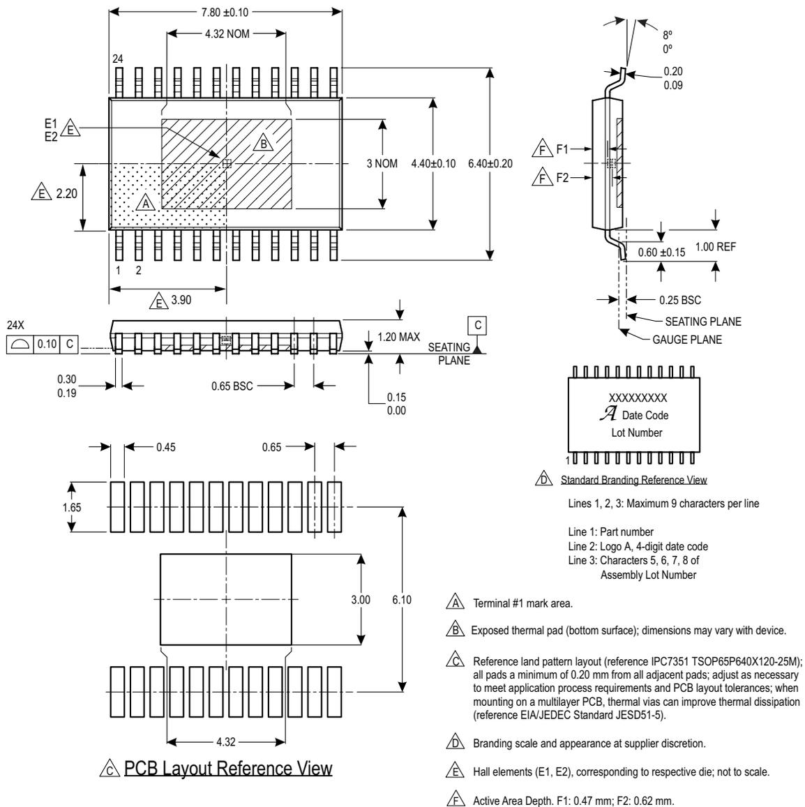
Figure 50: Package LP, 24-Pin TSSOP with Exposed Thermal Pad
