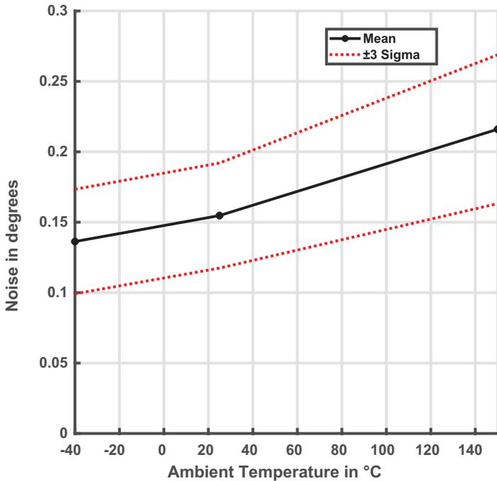
Figure 7: Noise Performance over Temperature (3 Sigma, 300 G)
