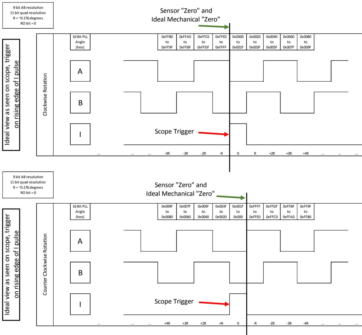
Figure 20: Index Pulse Corresponding to “Zero” Position
