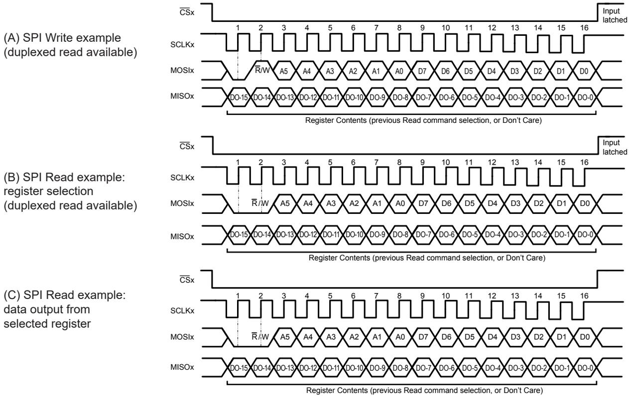
**Figure 33: SPI Read and Write Pulse Sequences**
