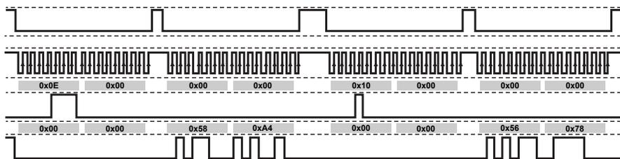
Note that it would have been possible to pipeline transactions in this example, i.e. send a new command while reading return data from the old command. This way the transaction could have been performed in 5 SPI frames instead of 8.
