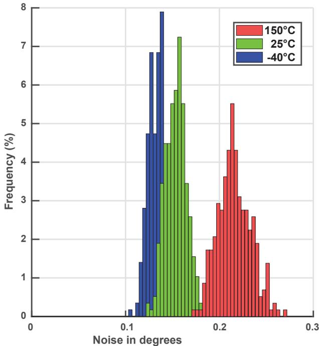
Figure 9: Noise Distribution over Temperature (3 Sigma, 300 G)
