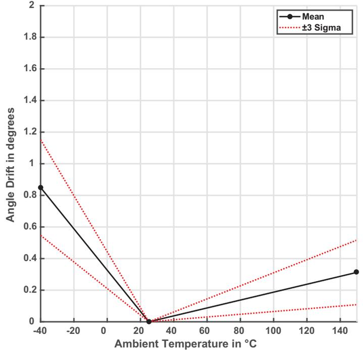
Figure 4: Maximum Absolute Drift from 25°C Reading (300 G)
