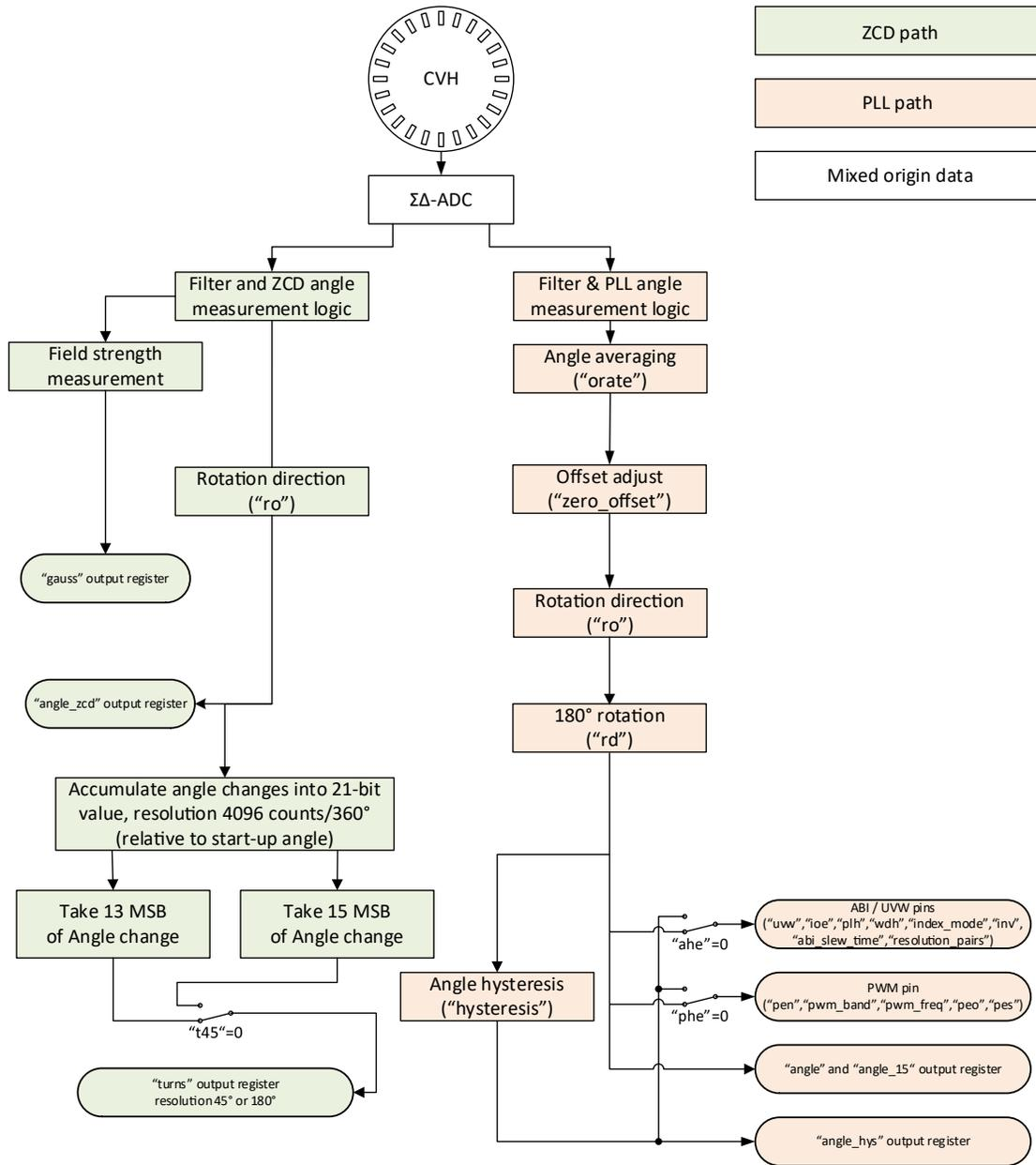
Figure 13: Angle Measurement – Sensor Readout Steps
