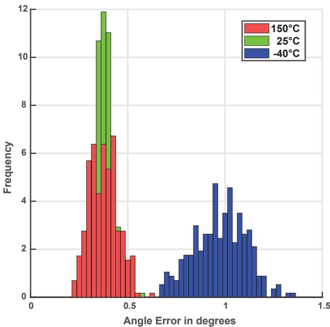
Figure 5: Peak Angle Error Distributions over Temperature (300 G)
