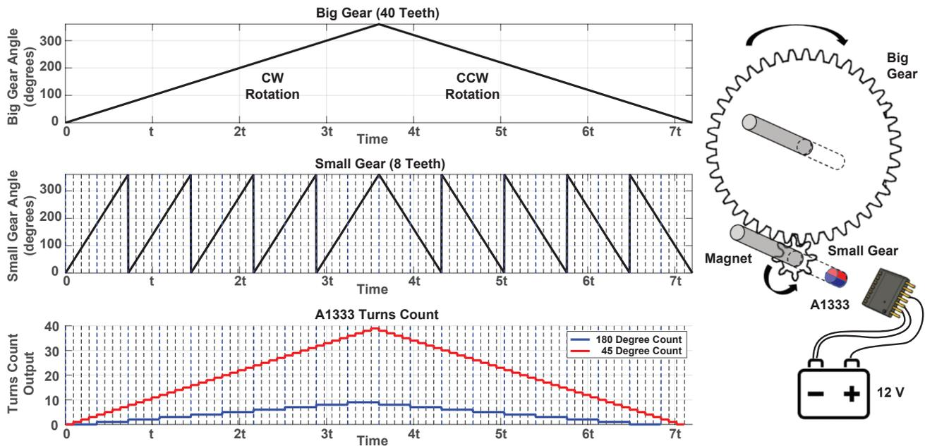
Figure 25: Example of a Turns Counting Application
