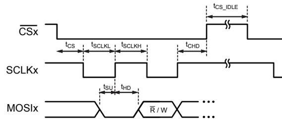
Figure 28: SPI Interface Timings Input
