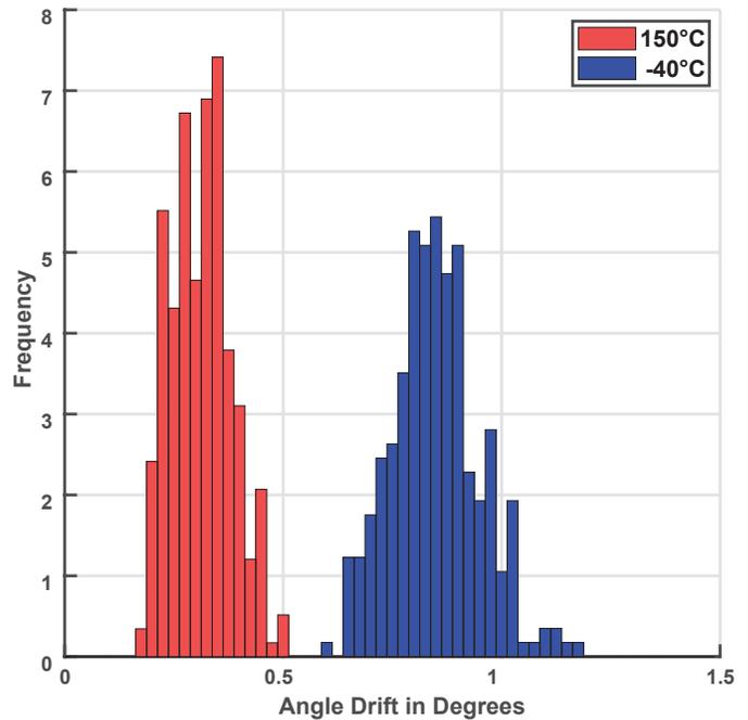
Figure 6: Angle Drift from 25°C (300 G)
