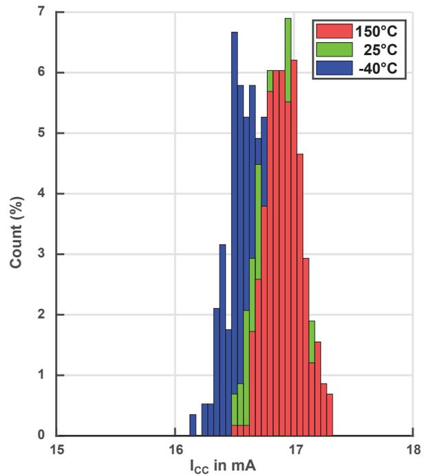
Figure 10: I<sub>CC</sub> Distribution over Temperature (V<sub>CC</sub> = 16.0 V)
