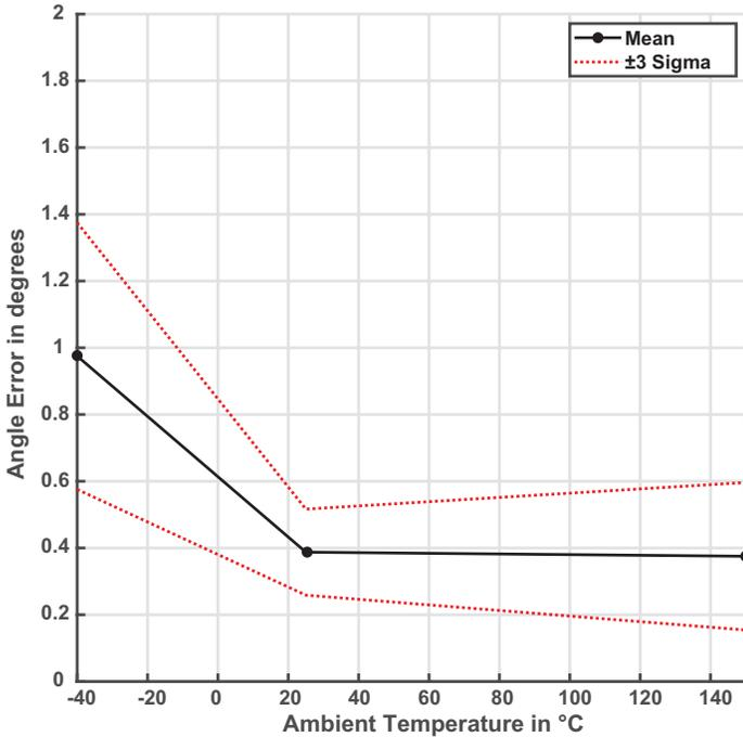
Figure 3: Peak Angle Error over Temperature (300 G)
