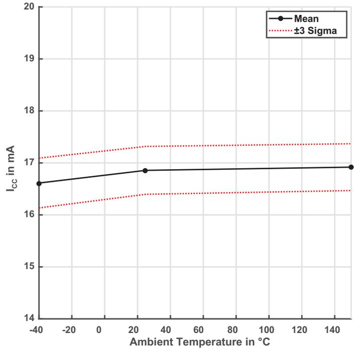
Figure 8: I<sub>CC</sub> over Temperature (V<sub>CC</sub> = 16.0 V)
