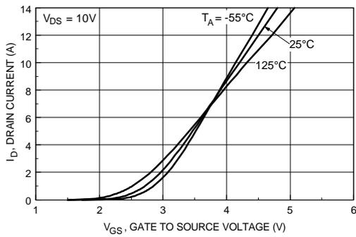
Figure 5. Transfer Characteristics.
