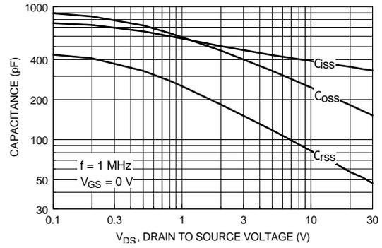
Figure 8. Capacitance Characteristics.
